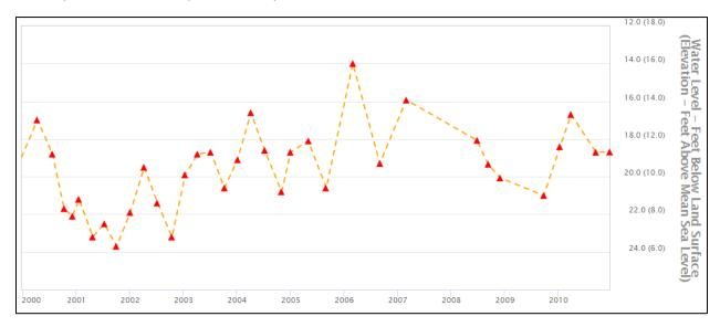
Figure 3. As shown, the groundwater elevation varied between 6.0 ft mean sea level (MSL) (10 ft MLLW) and 14.0 ft MSL (18 ft MLLW).
