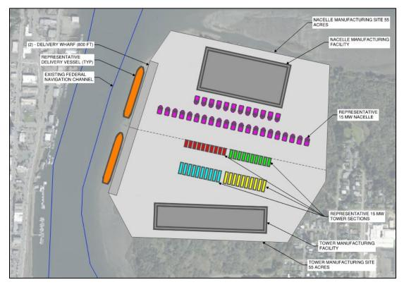
Figure 17. Tower and nacelle manufacturing site at Eastside Port Parcel
