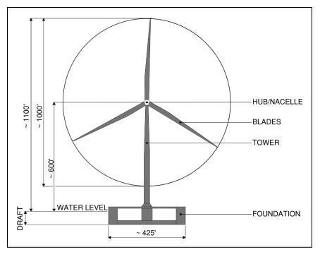
Figure ES.1. Floating offshore wind turbine dimensions
