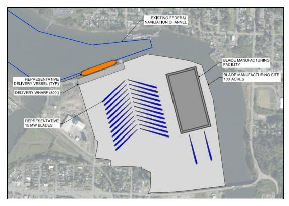
Figure 16. Blade manufacturing site at Terminal 1
