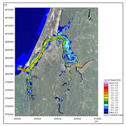
Figure 5. Maximum (99th percentile) depth-averaged currents for flood tides (USACE 2019)
