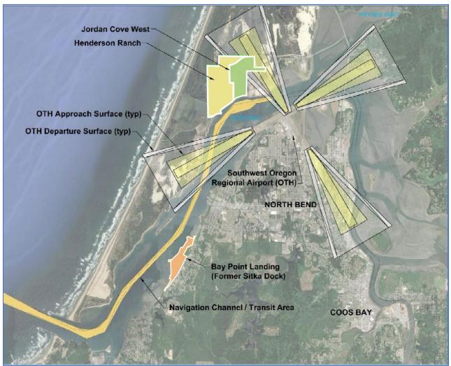
Only AC 150/15300-13B Section 3.6 large airplane surface 3, IFR circling surface 4, and instrument departure surface 7 shown in figure.
