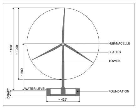
Figure 8. Floating offshore wind turbine dimensions
