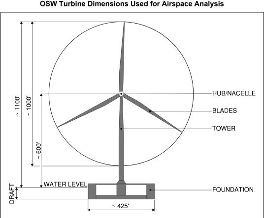
Figure 1: OSW Turbine Dimensions Used for Airspace Analysis
