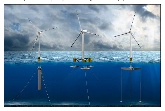
Figure 3. Illustration of floating foundation types (left to right: spar, semi-submersible, TLP) (NREL 2022)
