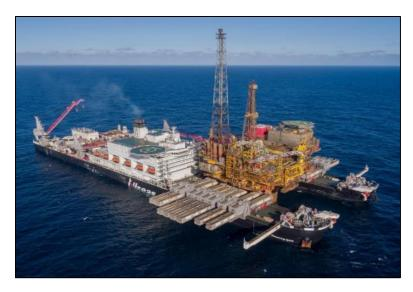
Figure 14. Pioneering Spirit transporting the Brent Delta topside (Shell 2019)
