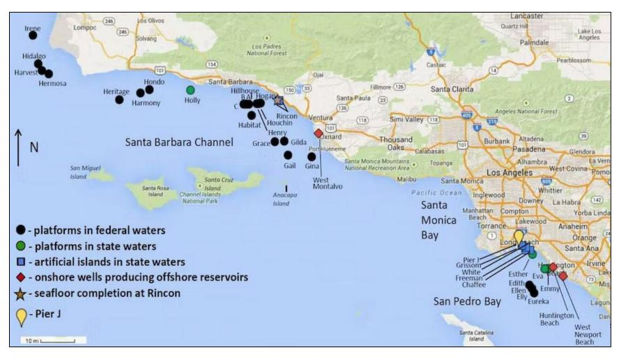
Figure 9. California offshore oil & gas platforms (CSLC 2018)
