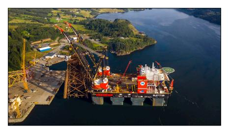
Figure 20. Sleipnir loading Brent Alpha's upper jacket onto the wharf at AFOD Facility in Norway (Heerema Marine Contractors)
