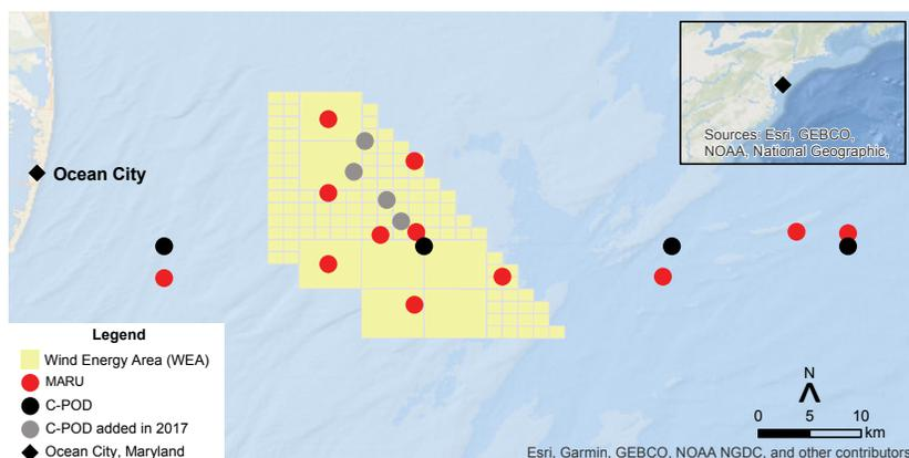
Underwater listening devices were deployed inside and outside the Maryland WEA. Twelve devices sensitive to the low-frequency calls of large whales (MARUs) were deployed throughout the WEA, inshore and offshore of the WEA (red circles). Four devices that can detect dolphin and porpoise clicks (C-PODs) were deployed in a transect line across the area studied (black circles) and a further four sites were added inside the WEA in 2017 (gray circles).
