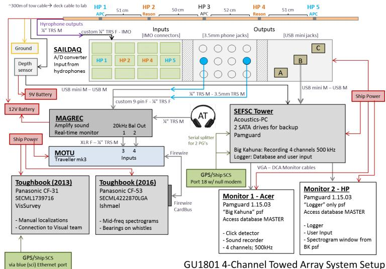
**Appendix A:** Acoustic setup diagram including towed hydrophone array, acoustic recording hardware, data inputs, and software.
