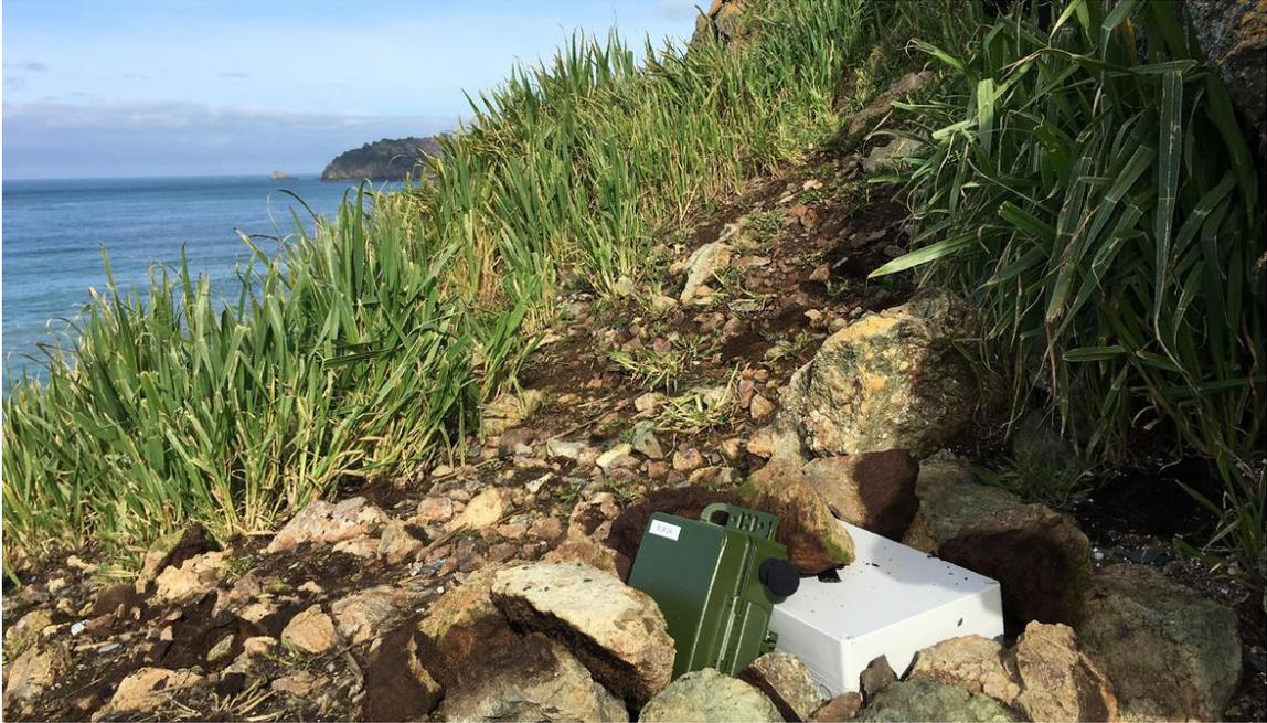
**Figure 6. Passive, digital acoustic recording unit**
