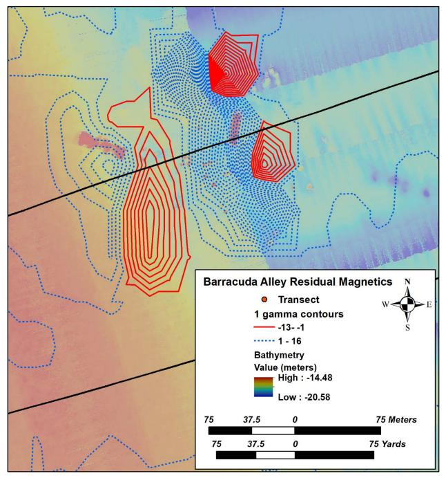
Figure 80. Detail of Barracuda Alley N1 survey area Residual magnetic contours overlaid multibeam echosounder bathymetry. Artificial Reef created by S.C Department of Natural Resources.
