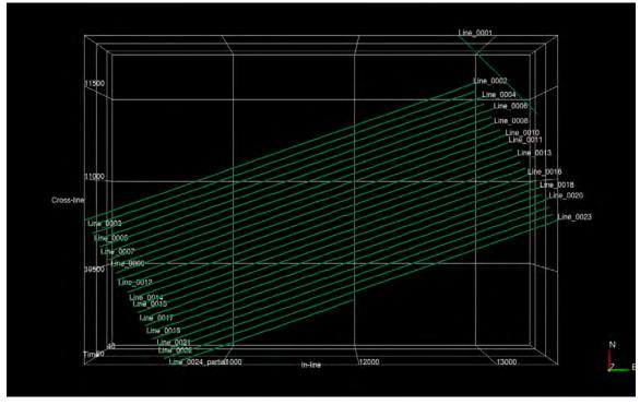
Figure 35. Map view of all the seismic lines collected in the target area
