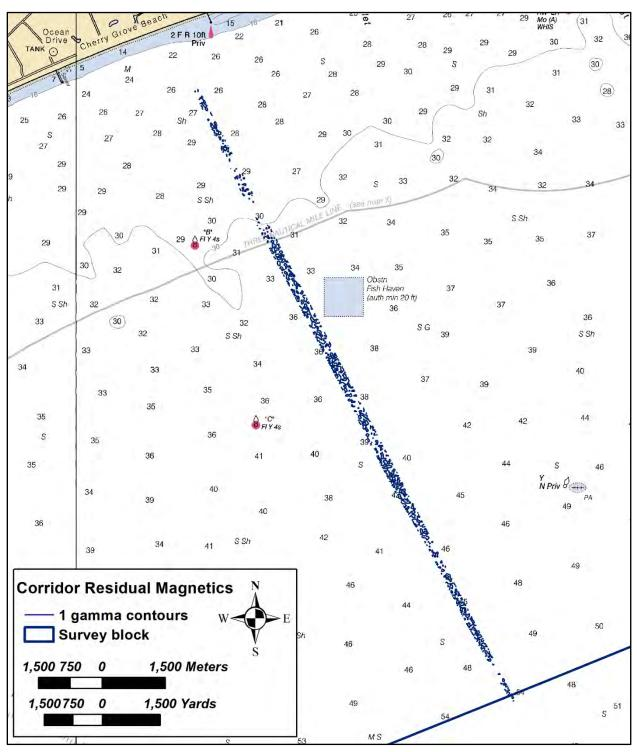
Figure 83. Residual magnetic contours of the Corridor survey area NOAA Nautical chart 11535, scale 1:80,000, 2018.
