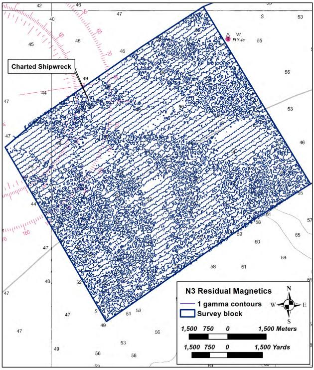
Figure 82. Residual magnetic contours of the N3 survey area NOAA nautical chart 11535, scale 1:80,000, 2018.
