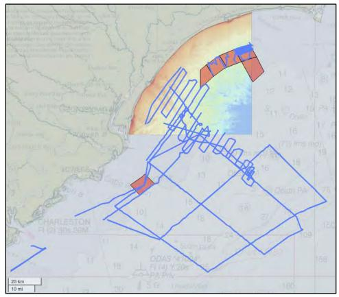
**Figure 10. CHIRP sub-bottom tracklines from the R/V** *Coastal Explorer* CHIRP sub-bottom tracklines from the R/V *Coastal Explorer* (northern Long Bay, grouped red polygons) and the R/V *Nancy Foster* (large grid of southern Long Bay).
