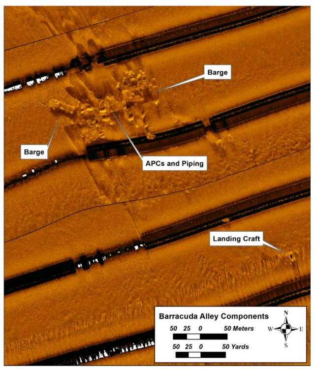
Figure 79. Detail of side-scan sonar coverage of Barracuda Alley in N1 survey area Artificial Reef created by S.C. Department of Natural Resources.
