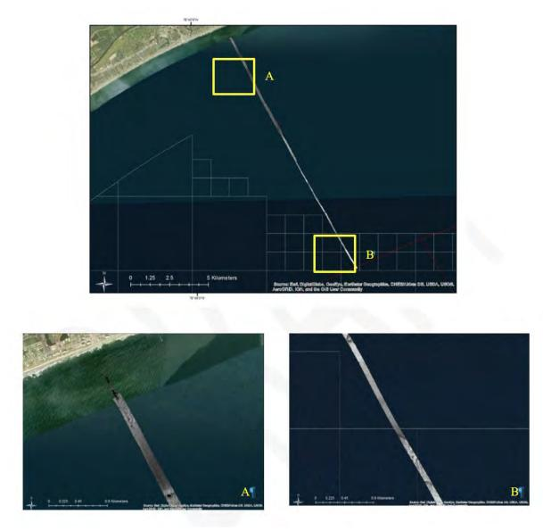
**Figure 97. Seafloor sonar backscatter mosaic of the representative cable corridor** A and B enlargements of the innershore and offshore areas better illustrating the backscatter patterns.
