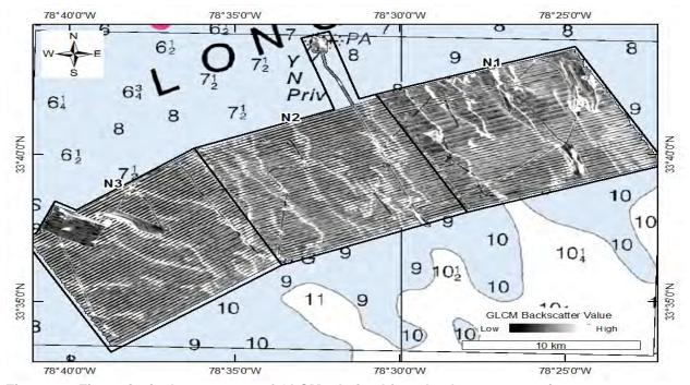
**Figure 21. First principal component of GLCMs derived from backscatter mosaic** The three GLCMs used to describe seafloor texture are homogeneity, second moment, and entropy. Ridges and ripples are clearly visible in the resulting textural image.
