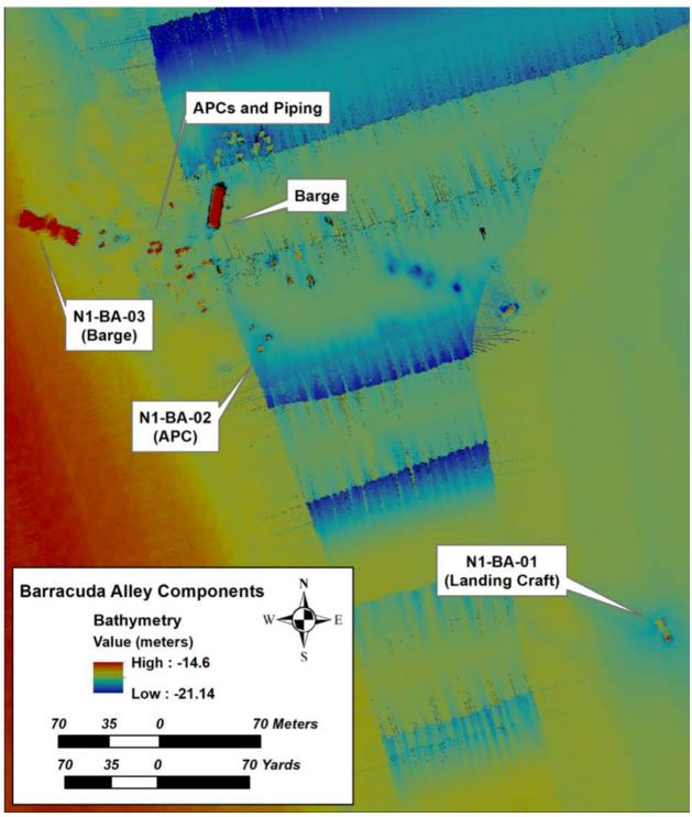
Figure 87. Detail of multibeam echosounder coverage of Barracuda Alley in N1 survey area Artificial Reef created by S.C. Department of Natural Resources.
