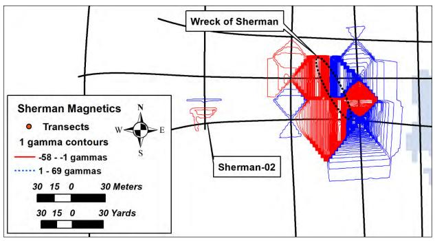
Figure 84. Residual magnetic contours of the wreck of *Sherman* and environs NOAA nautical chart 11536, scale 1:80,000, 2018.
