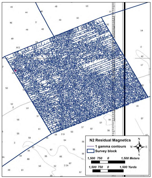
Figure 81. Residual magnetic contours of the N2 survey area NOAA nautical chart 11535, scale 1:80,000, 2018.
