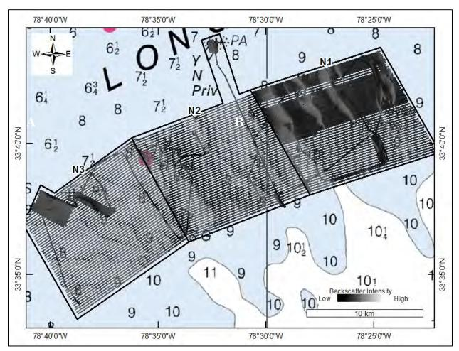
**Figure 15.** Backscatter coverage of the concession area Backscatter mosaicked at a 0.5 m grid. Light-colored features indicate sonar sounding returns of high intensity. Highintensity returns can occur on hardbottom surfaces and shallow features that are closer to the sonar receiver.
