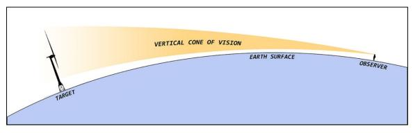
Figure 1. Effect of Earth Curvature on Visibility
