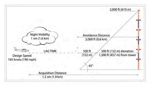
Figure B-1. Illustration of Acquisition Distance Calculation
