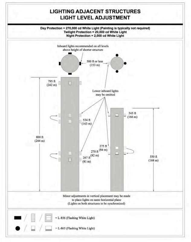
Figure A-18. Lighting Adjacent Structures—Light Level Adjustment
