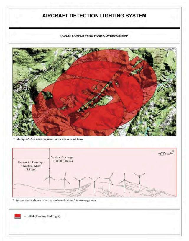
Figure A-27. Sample of Aircraft Detection Lighting System Coverage Map
