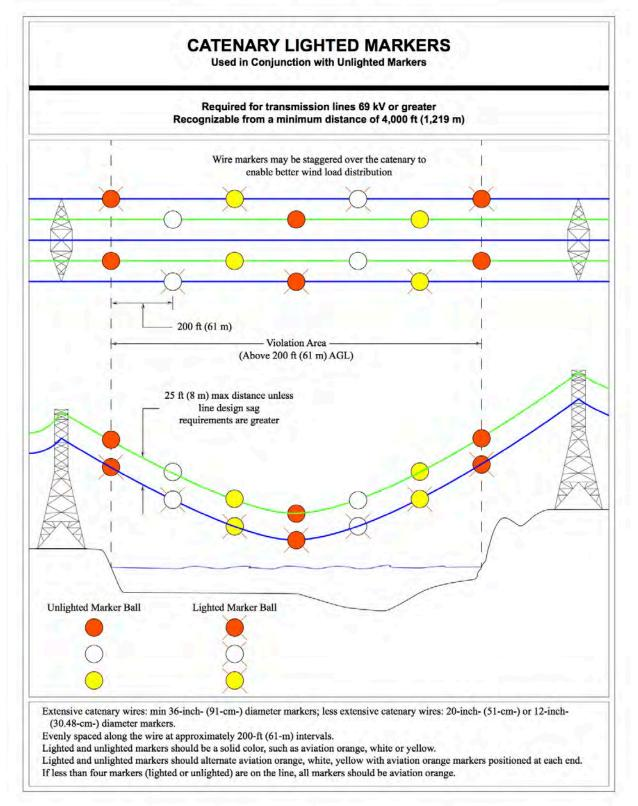
Figure A-5. Catenary Lighted Markers Figure A-5. Catenary Lighted Markers
