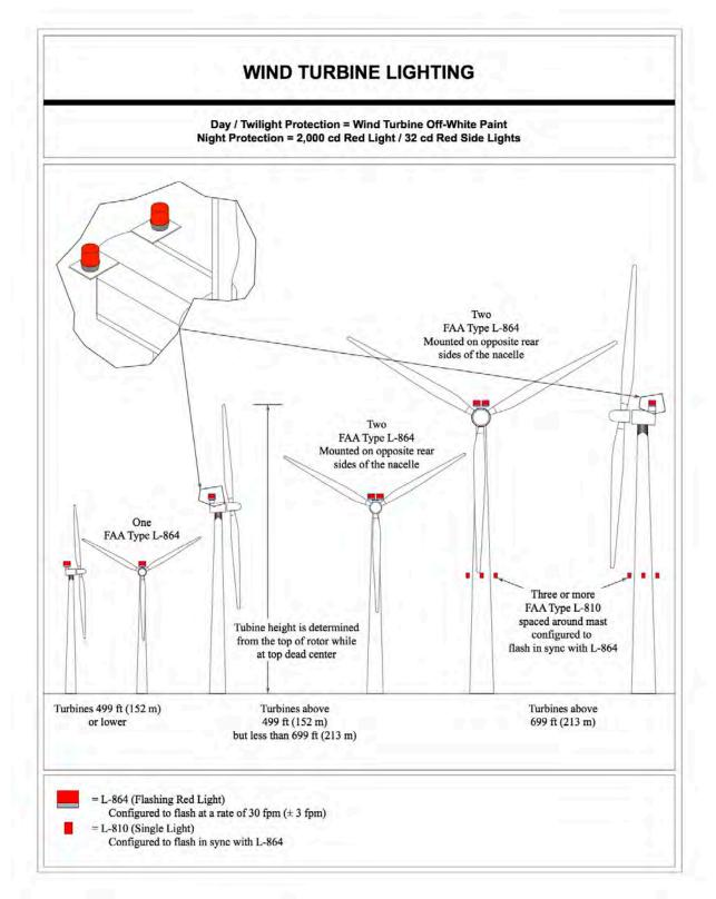
Figure A-23. Wind Turbine Lighting
