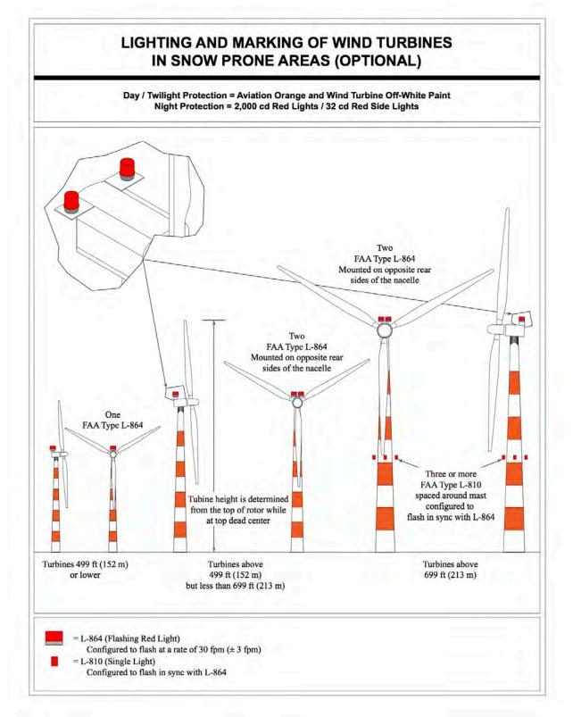
Figure A-24. Wind Turbine Lighting and Marking in Snow Prone Areas (Optional)
