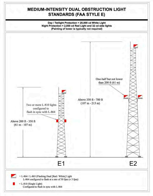
Figure A-10. Medium-Intensity Dual Obstruction Lighting Standards
