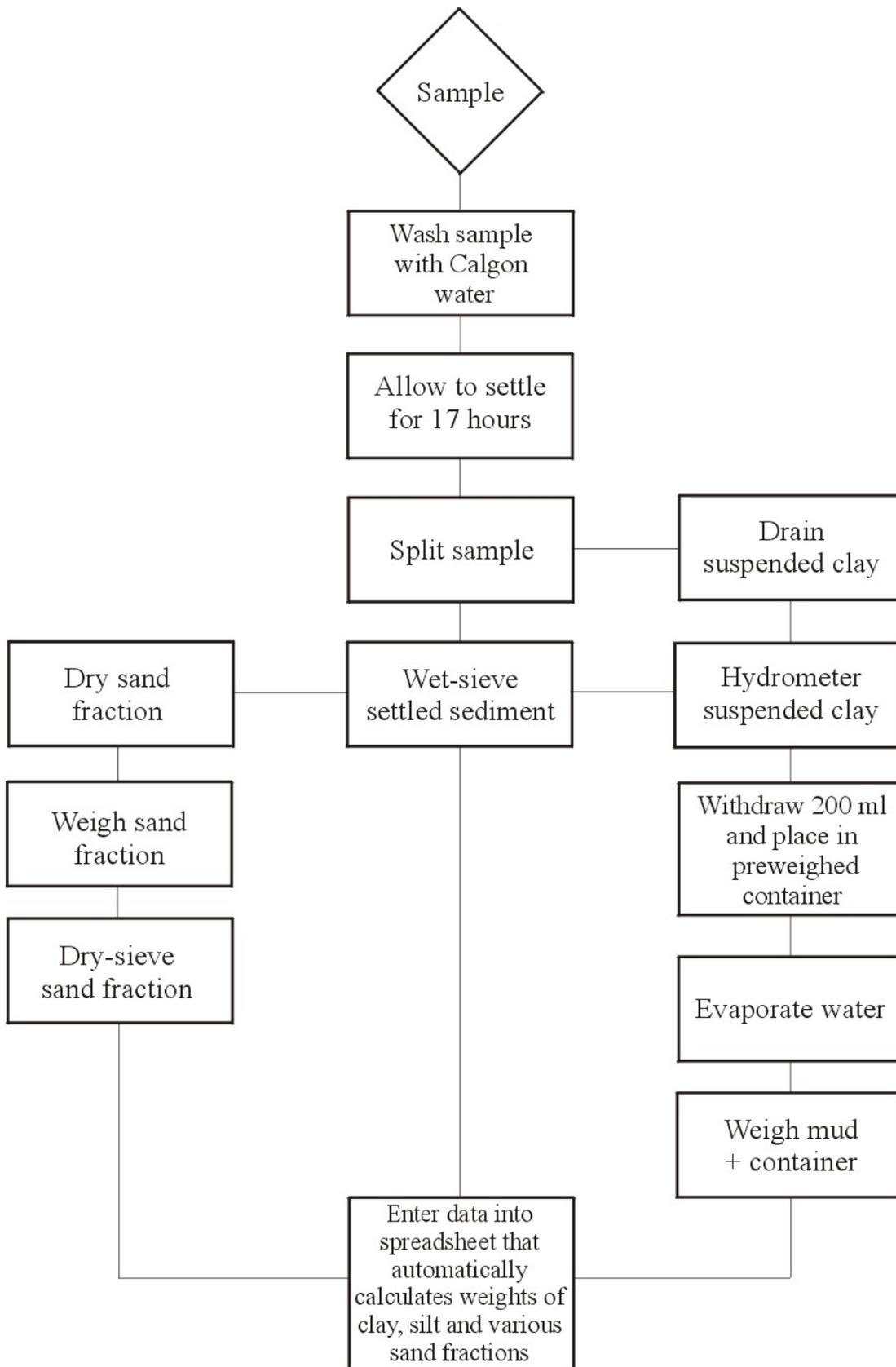
Figure 3. Flow chart for particle-size analysis.
