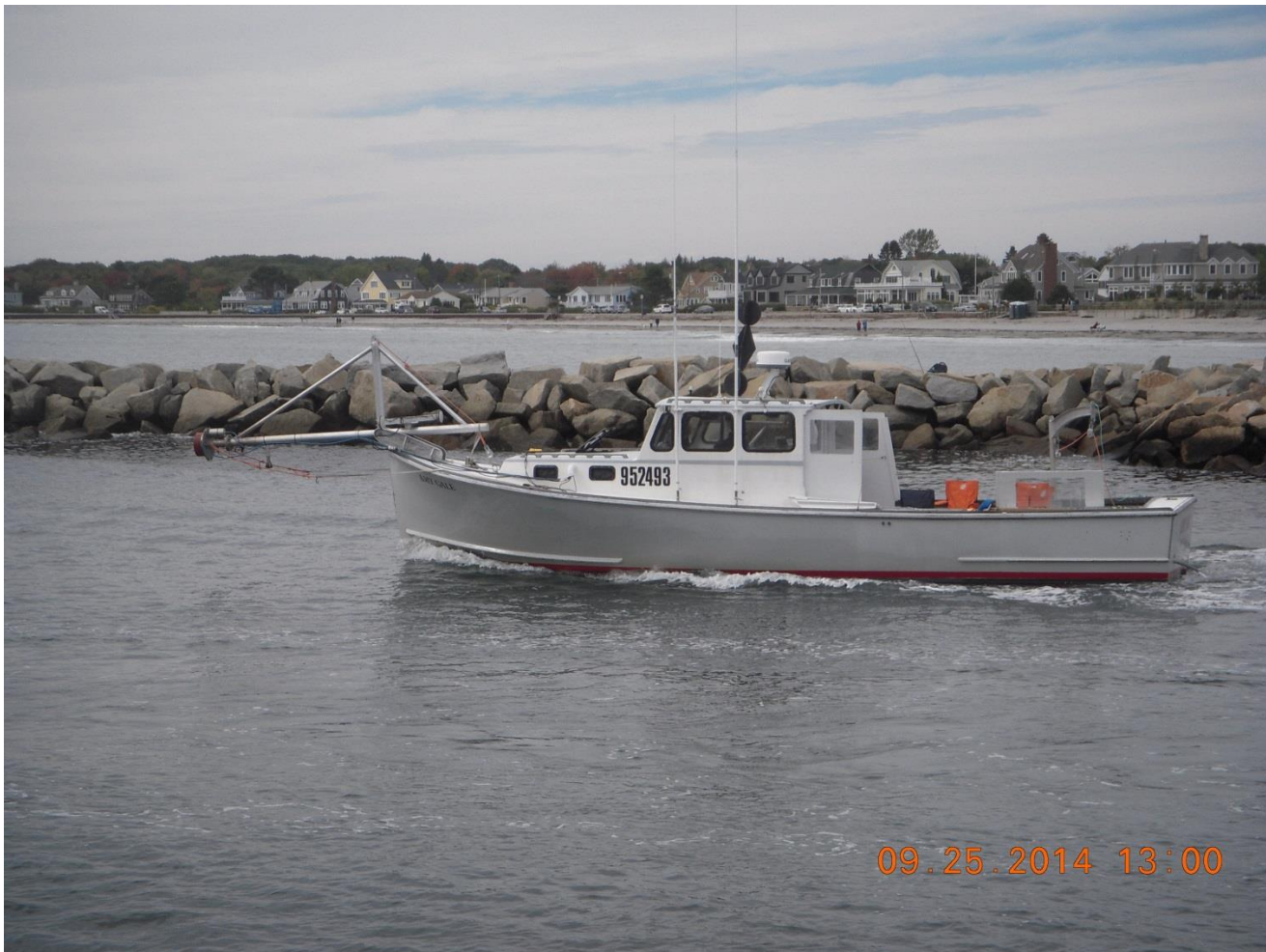
Figure 2: F/V Amy Gale, with bow mounted transducer, MRU and antennas.
