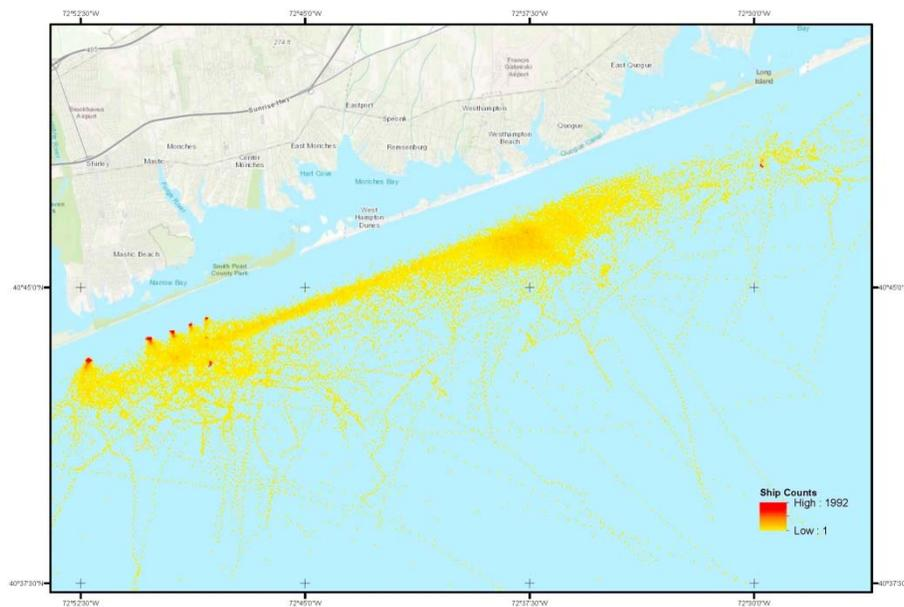
Figure 4. Heat map of dredge positions. The dredged area is represented by the warm colors to the right while the discharge locations are represented by the five reddish areas to the left
