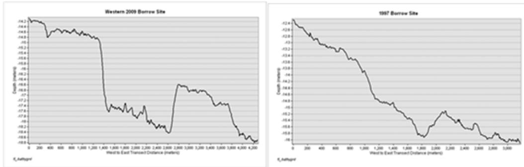
**Figure 3. a. 2011 survey of the CP&E Western Borrow Area which had been dredged in 2009. b. 2011 survey of the Fire Island Pines Borrow Area which had been dredged in 1997.**
