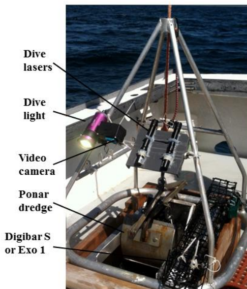
Figure 2. MCMC grab sampling platform.
