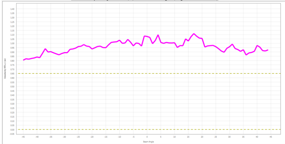
Uncertainty: Depth Bias (% of water depth) vs. Beam Angle (degrees from nadir)
