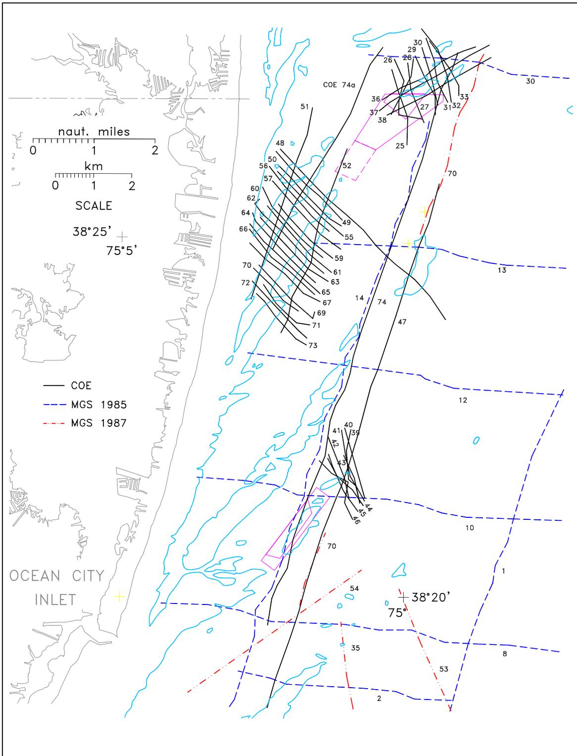
**Figure 6.** Track lines for high-resolution seismic profiles collected by the U.S. Army Corps of Engineers (COE) in 1986 (black solid lines). Also shown are selected track lines of seismic profiles collected by the Maryland Geological Survey in 1985 (blue dashed lines) and in 1987 (red dot-dashed lines). The 10-meter isobath (light blue) and borrow areas 2 and 3 boundaries (purple lines) are indicated for reference.
