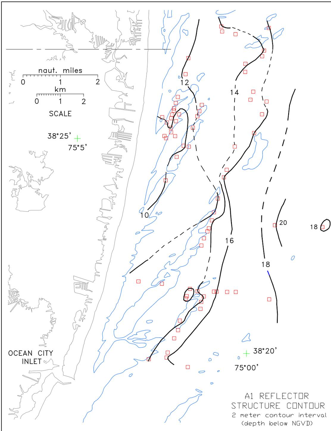
**Figure 13.** Structure contour of the A1 reflector. Red squares indicate data points. Depths to the A1 reflector were taken primarily from ORE 3.5 kHz seismic records. The A1 reflector is discontinuous, absent in the trough areas where the underlying depositional units are exposed. These areas are indicated by dashed structure contours. The contour interval is 2 meters (below NGVD).
