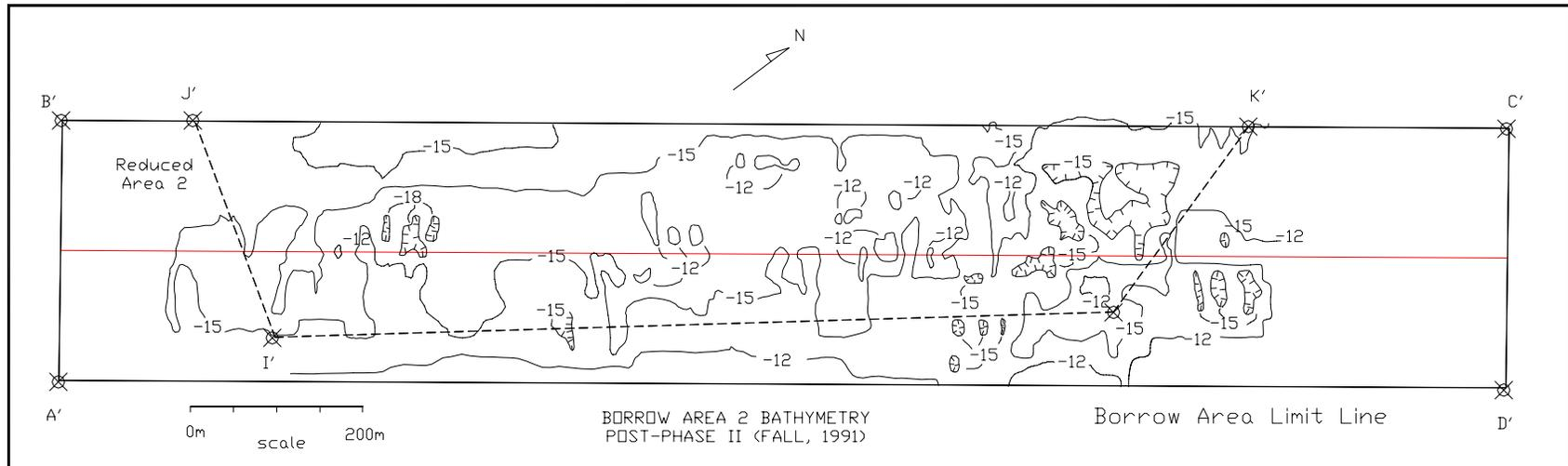
**Figure 18.** Pre- and post-dredging bathymetry of borrow area 2. Location of the cross-section shown in Figure 19 is indicated by a red line bisecting the borrow area
