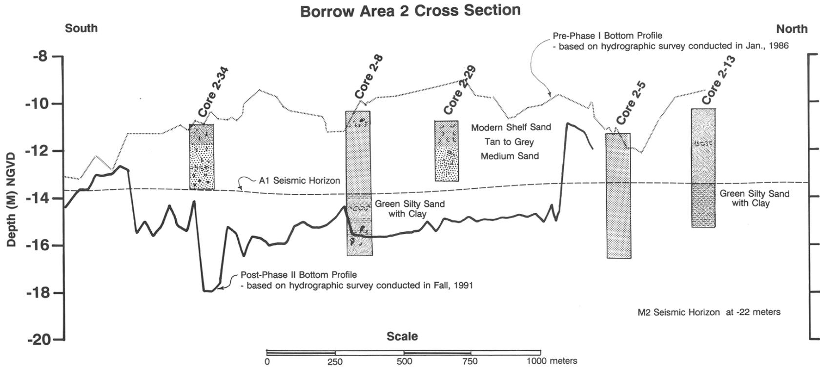
**Figure 19.** Cross-section of borrow area 2 illustrating pre- and post-dredging surfaces relative to mapped seismic horizon (A1) and lithologic changes.
