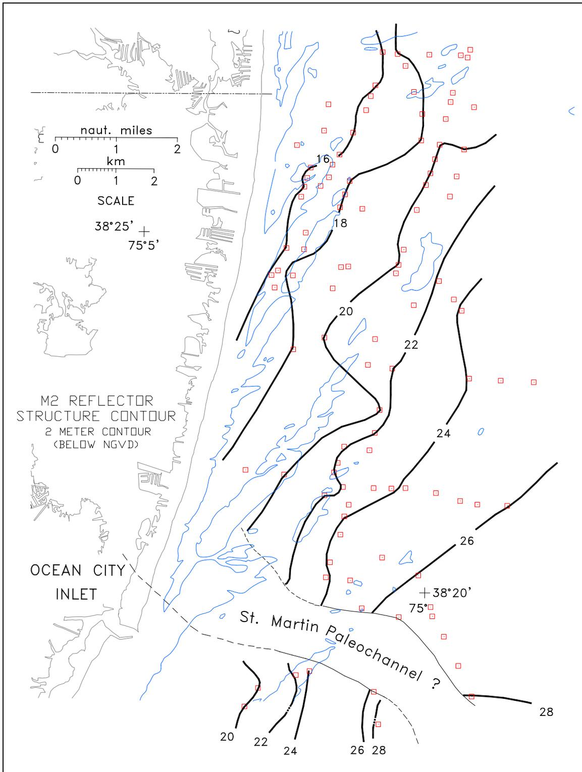
**Figure 9.** Structure contour of M2 reflector. Open squares (red) indicate data. Depths to the M2 reflector were taken primarily from ORE 3.5 kHz seismic records. The contour interval is 2 meters (below NGVD). The 10-meter isobath (blue lines) is shown for reference.
