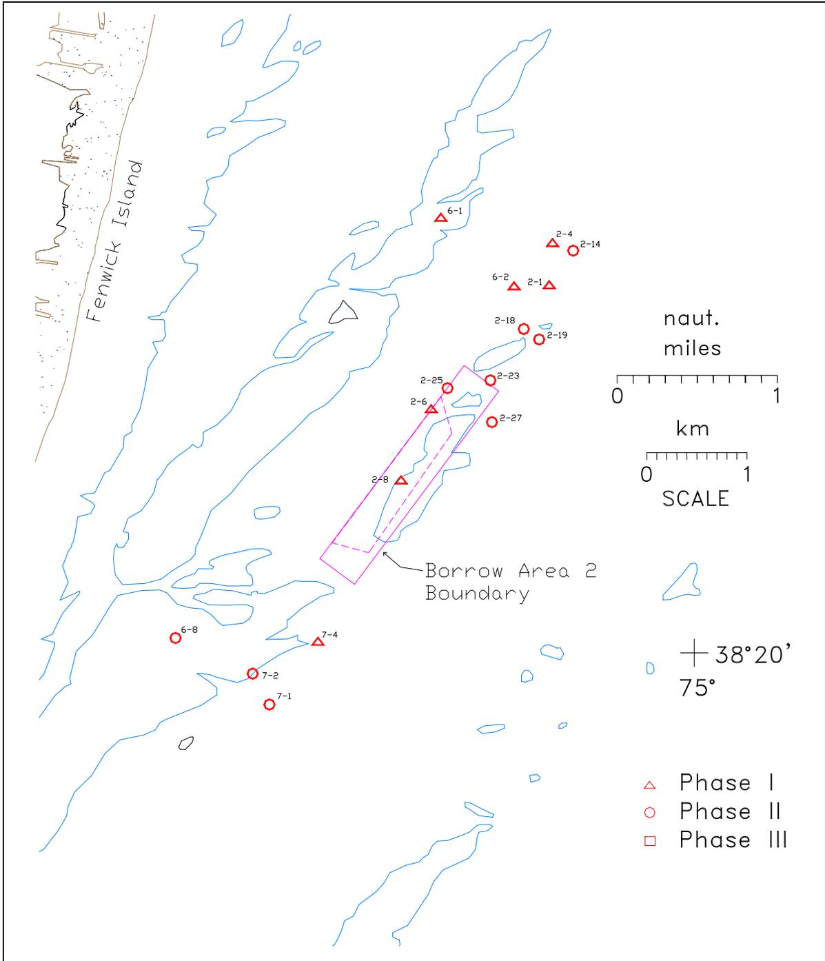
**Figure 16.** Shoal 2 vicinity detailing borrow area dredging limits and selected core locations. The State contract (Phase I) dredging area is indicated by the dashed lines within borrow area. The cores shown are discussed in the text.
