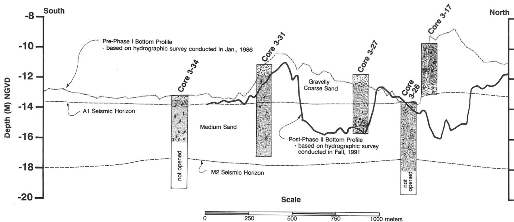
**Figure 21.** Cross-section of borrow area 3 illustrating pre- and post-dredging surfaces relative to the A1 horizon and lithologic changes.
