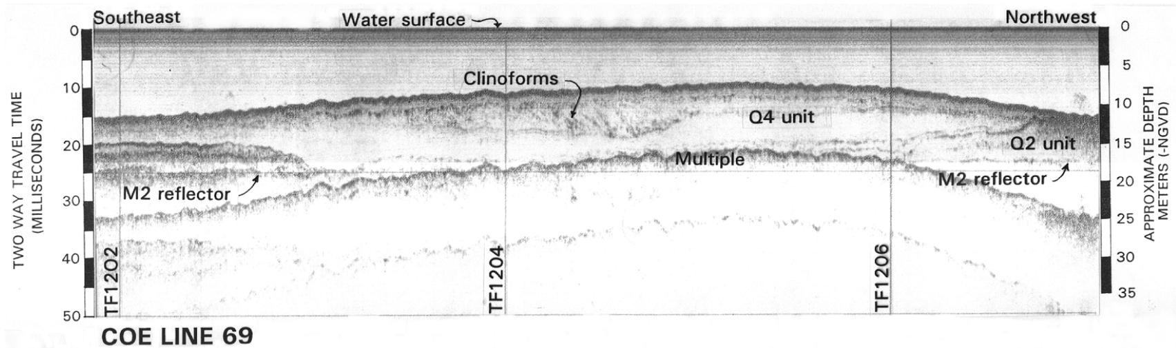
**Figure 12.** Section of seismic record (ORE 3.5 kHz) for COE line 69. This seismic record crosses shoal 4 and features a broad paleochannel incised in the underlying Q2 (see Plate 3 for interpreted profile). Internal reflectors show several episodes of cut and fill. Fill features in the shallower channel suggest clinofolds. The shallow channel is interpreted to be a laterally aggrading channel, either tidal or inlet related.
