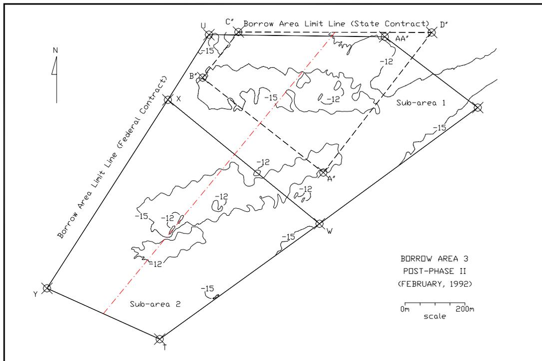
**Figure 20.** Pre- and post-dredging bathymetry for borrow area 3. Location of the cross-section shown in Figure 21 is indicated by a red dashed-dot line bisecting the borrow area.
