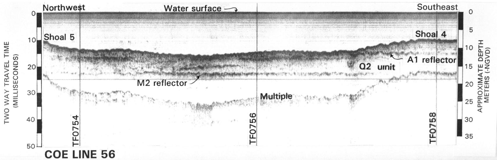
**Figure 8.** Section of seismic record (ORE 3.5 kHz) for COE line 56. The M2 reflector is very prominent in the inter-shoal areas and attenuates beneath the shoals. Refer to Plate 1 for interpretation of entire profile line.
