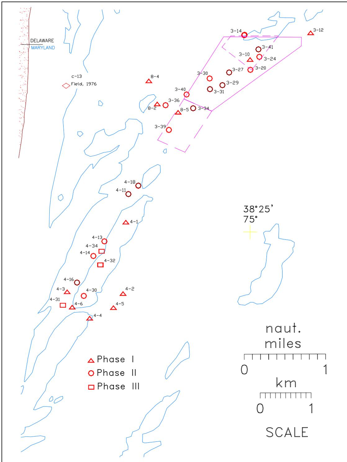
**Figure 17.** Shoals 3 and 4 and vicinity detailing borrow area dredging limits and selected core locations. The subarea shown within the north end of the borrow area was dredged during Phase I (State contract). Sub-area 3-III, indicated by the dashed lines at the southwest end of the borrow area, was dredged in the summer of 1992 for sand to repair storm damages in Ocean City. The cores shown are discussed in the text.
