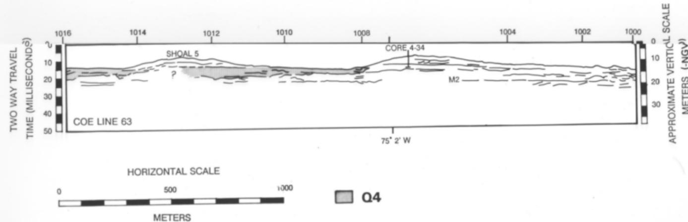
**Plate 2. Interpreted seismic profile lines COE 64, 65, 66, and 67 (ORE 3.5 kHz) collected on shoals 4 & 5. Acoustic units interpreted as Q4 deposits are indicated by gray shading.**
