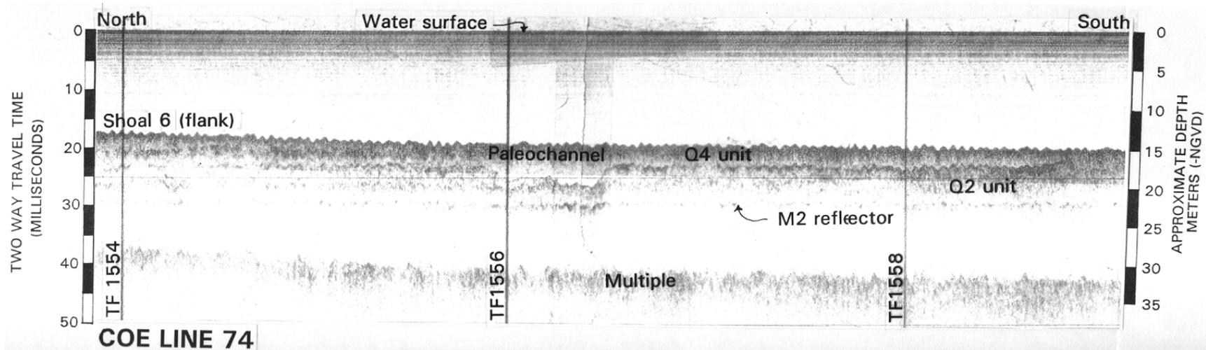
**Figure 10.** Section of seismic record (ORE 3.5 kHz) for COE line 74 featuring a broad shallow paleochannel. This paleochannel extends under shoal 6 west of the track line.
