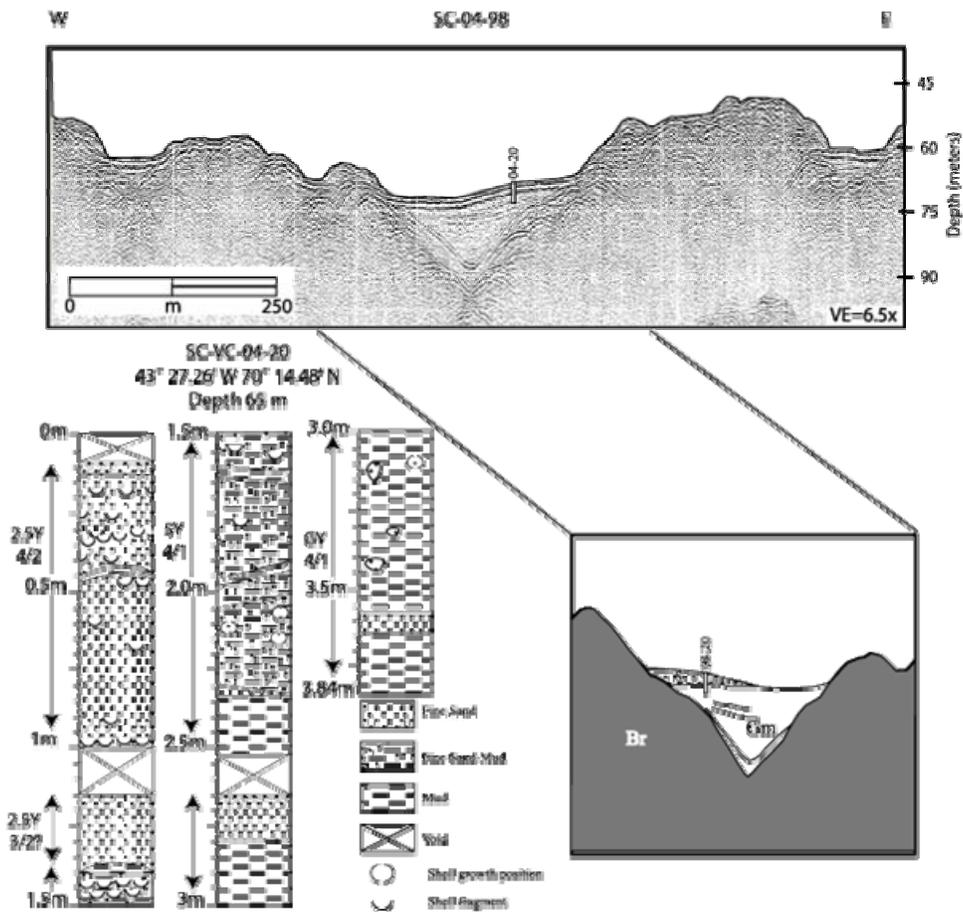
Figure 16. SCVC04-20 from Basin 6. All interpreted seismic units are the same as described in Figure 9.
