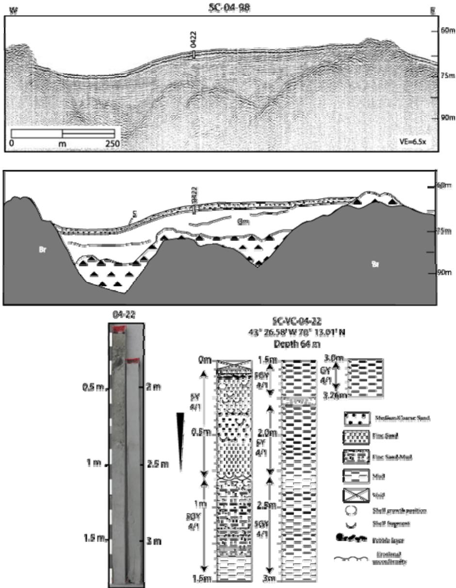
Figure 10. Vibracore SCVC04-22 collected along seismic line SC-04-98.
