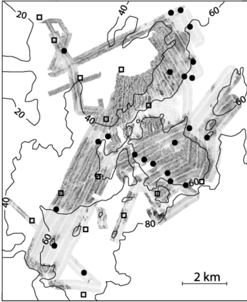
Figure 5. Side scan sonar mosaic of study area. Filled circles represent vibracore sites; open squares represent bottom samples collected earlier (Kelley et al., 1986b).
