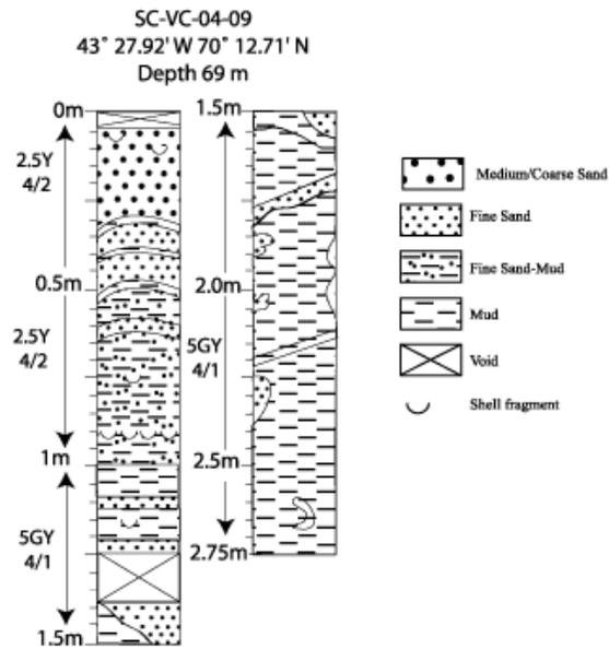
Figure 14. Core SCVC04-09 was collected in Basin 4 at about 65 m depth. All interpreted seismic units are the same as described in Figure 9.
