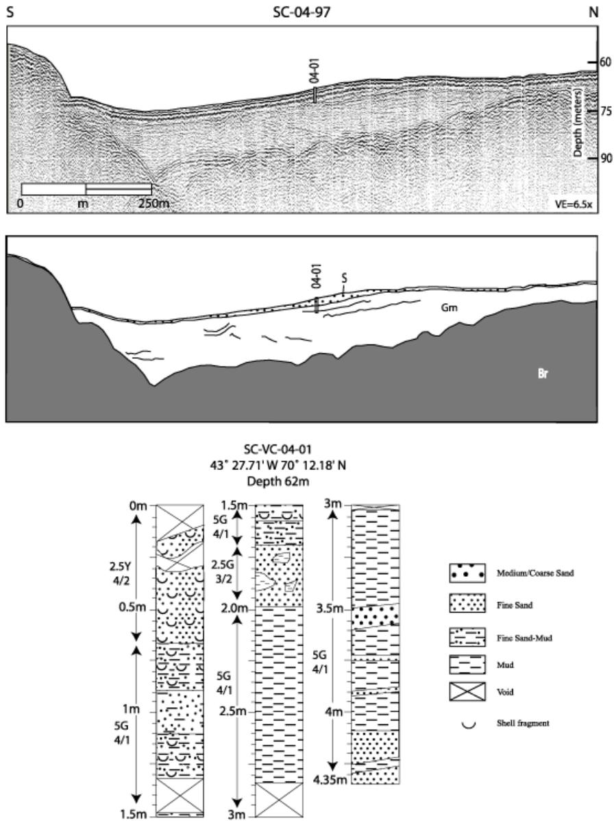
Figure 13. Core SCVC04-01 from Basin 3. All interpreted seismic units are the same as described in Figure 9.
