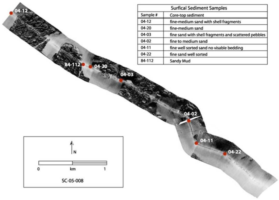
Figure 6. Detailed side scan sonar image of rock and gravel. The linear acoustic noise to either side of the center trackline was caused by ship heave in rough seas. Lighter tones represent ‘soft’ returns from mud; darker tones are “harder” returns from rock, sand and gravel. Side scan image is located in Figure 2.
