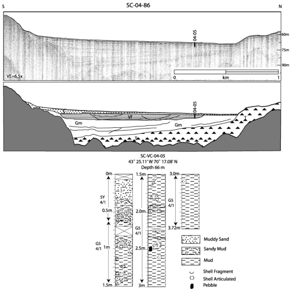
Figure 9. SRP and core from Basin 1. BR is bedrock, T is till, GM is glacial-marine mud, Vf is valley fill, S is sand.
