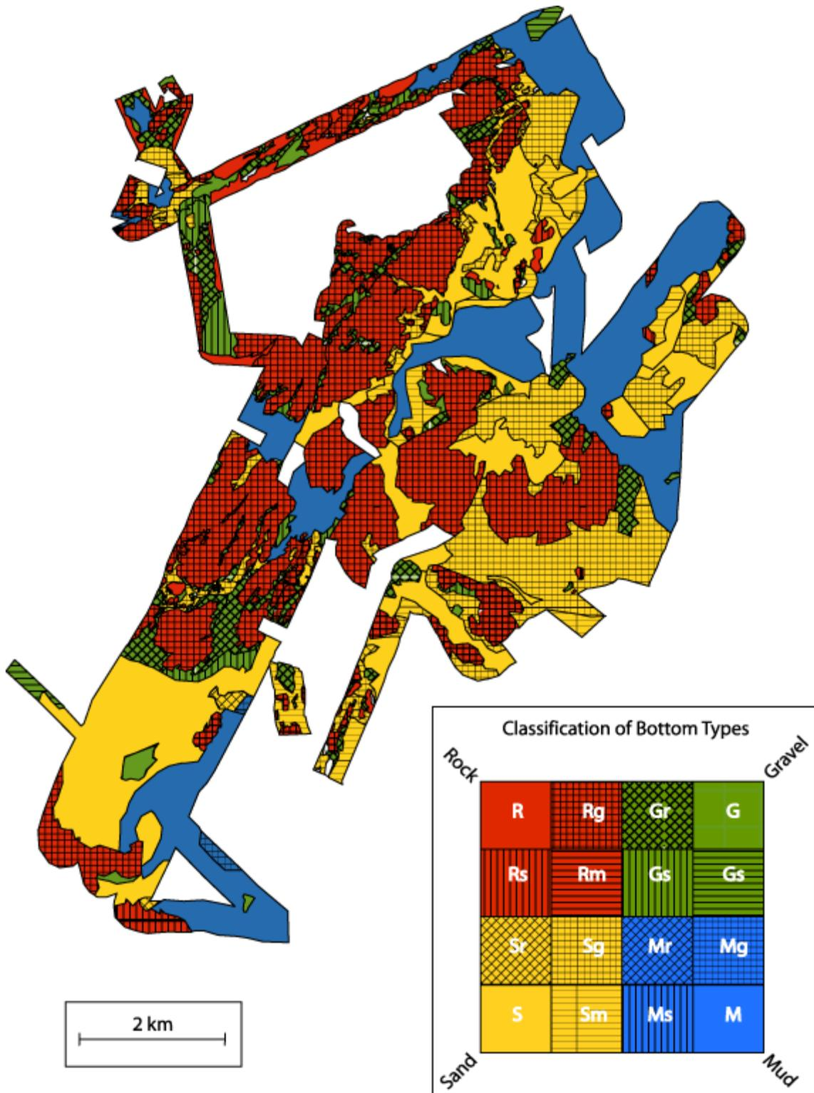
Figure 8. Surficial material map interpreted from side scan sonar, and bottom and core samples.
