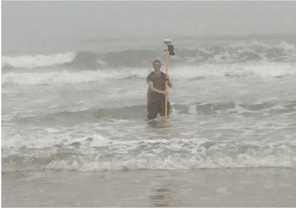
Figure 2. Doug Beach measuring beach profiles on Plum Island in March 2016 with a Real Time Kinematic Trimble R8 Global Navigation Satellite System linked to the cellular phone network.
