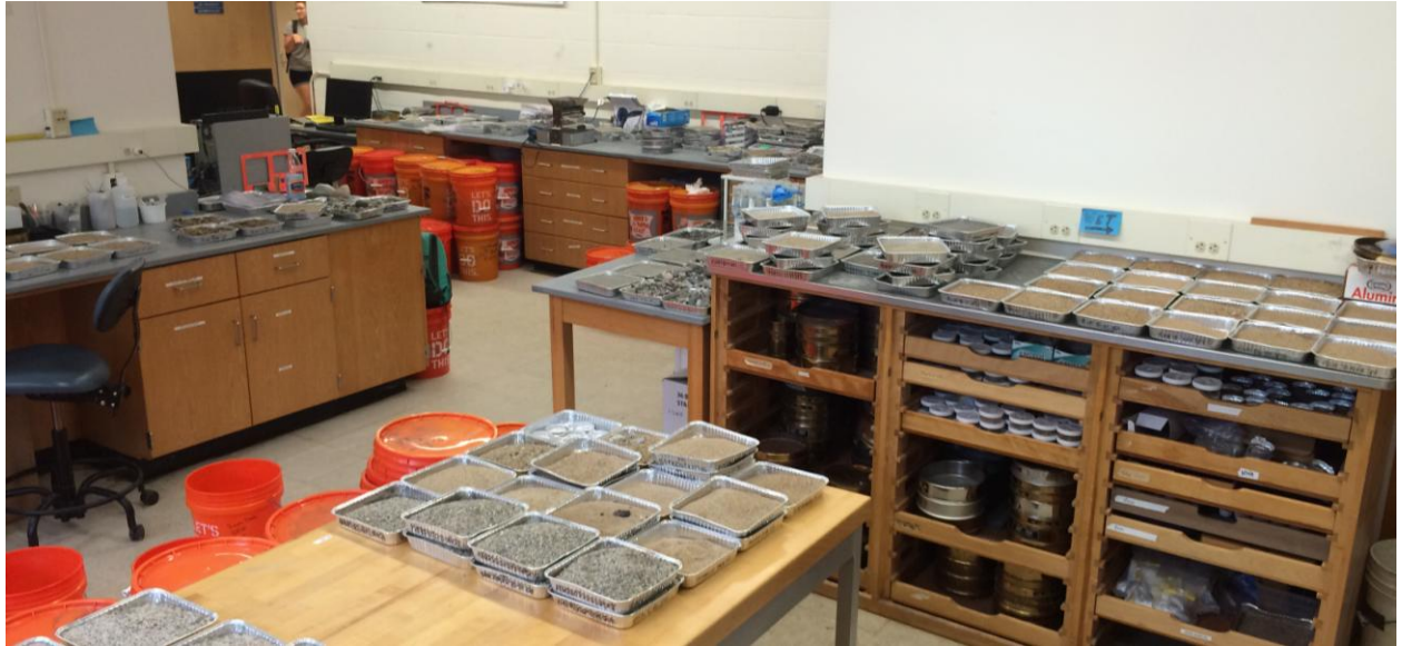
Figure 1. Picture from the University of Massachusetts Amherst sedimentology lab showing samples in pans in preparation for weighing and sieving for the greater than 4 mm fraction.
