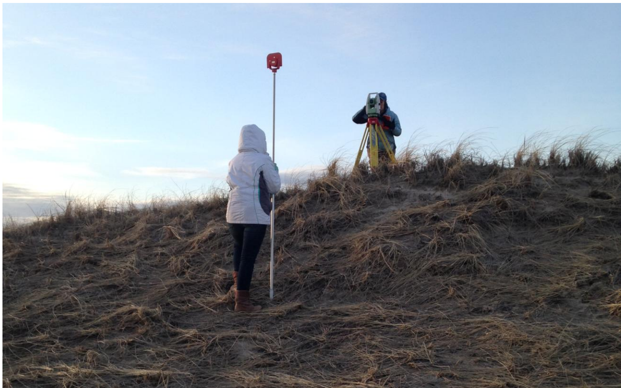
Figure 1. Jon Woodruff and Jen Journack measuring beach profiles with a Topcon GTS 210 total station on Miacomet Beach, Nantucket, March 2015.
