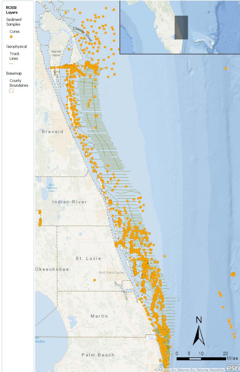
Figure 2. Brevard County to Palm Beach County portion of data (available through the Regional Offshore Sand Source Inventory MapViewer page <http://rossi.urs-tally.com/Map/>). The zig-zag track lines along the coastline reflect “chirp” data collection. The rectilinear track lines further offshore reflect “boomer” data collection.
