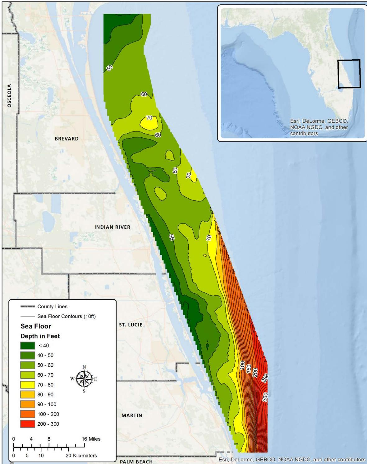
Figure 8. Bathymetric map of the seafloor south of Cape Canaveral based on boomer data collected from 1996 to 2000.
