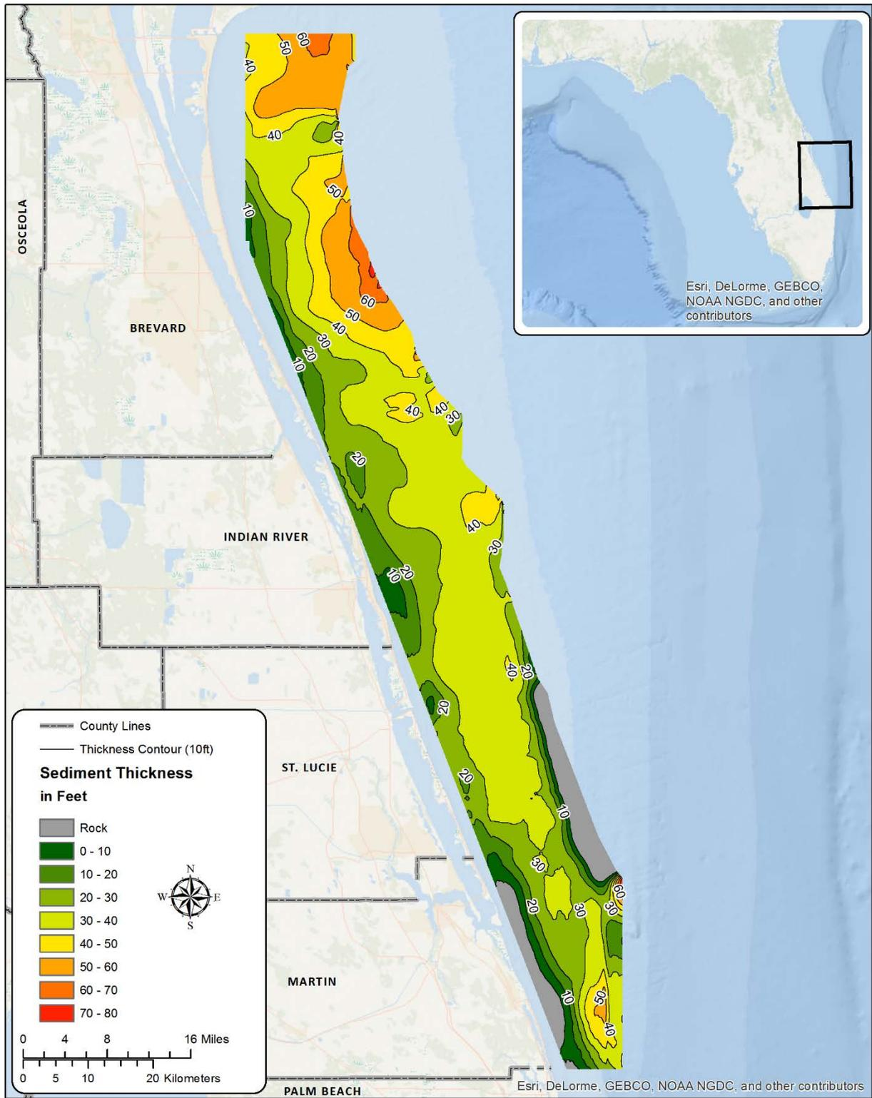
Figure 10. Unconsolidated sediment thickness south of Cape Canaveral based on boomer and chirp data, collected from 1996 to 2000, and 2007, respectively.
