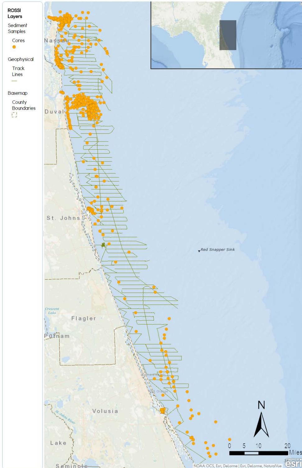
Figure 1. Nassau County to Volusia County portion of data (available through the Regional Offshore Sand Source Inventory MapViewer page <http://rossi.urs-tally.com/Map>). The zig-zag track lines along the coastline reflect “chirp” data collection. The rectilinear track lines further offshore reflect “boomer” data collection.
