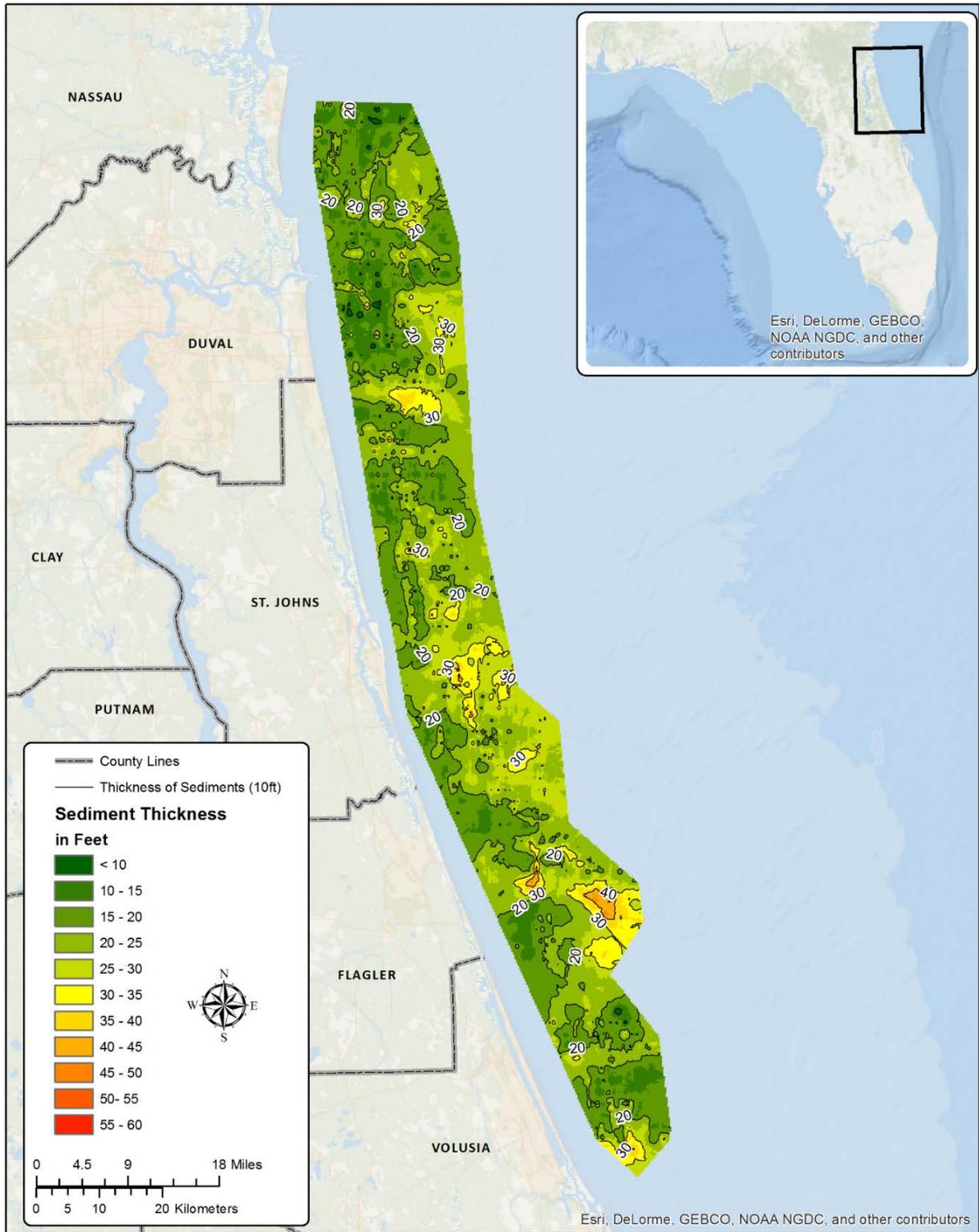
Figure 7. Unconsolidated sediment thickness north of Cape Canaveral based on boomer and chirp data, collected from 2002 to 2006, and 2007, respectively.
