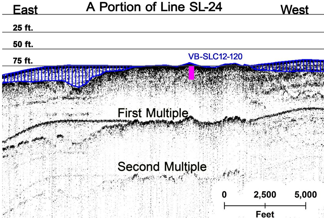
Figure 3. Seismic line SL-24 and vibracore VB-SLC12-120. The uppermost blue line delineates the seafloor, the lowermost blue line delineates the top of rock, and the thickness of unconsolidated sediments lying between those blue lines is illustrated by the vertical blue “hatch” lines.
