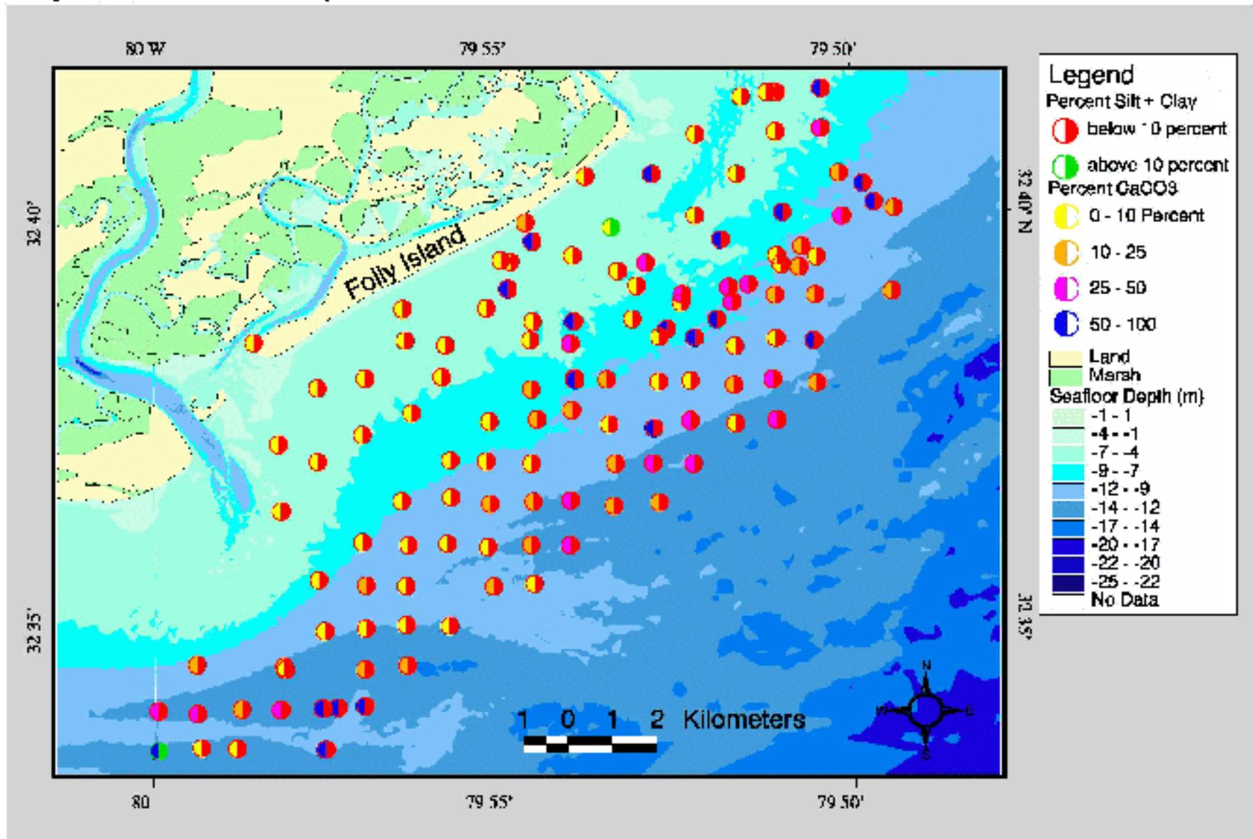
Figure 15. Percent silt/clay and percent carbonate values for surficial sediment samples from the inner shelf off Folly Island, South Carolina.
