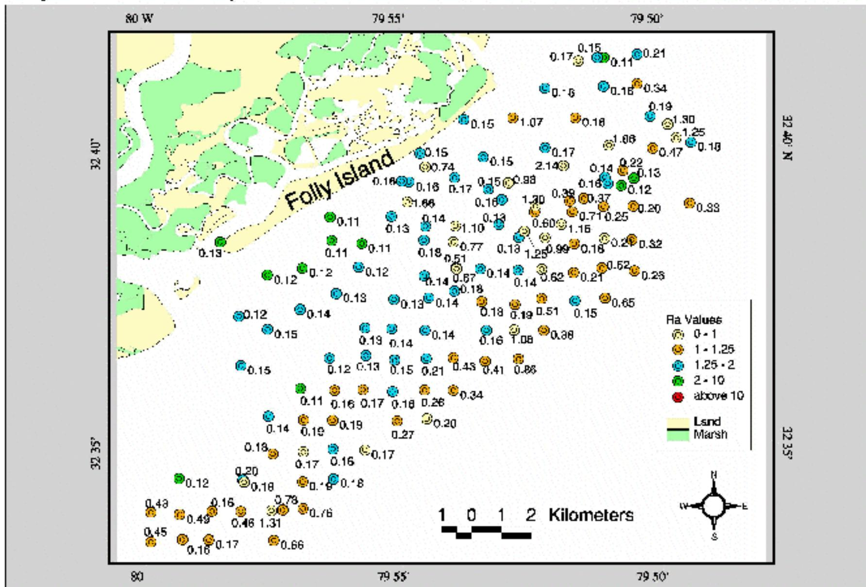
Figure 19. Surficial sediment sample mean grain size (mm) and Ra values (overfill ratio) for the inner shelf off Folly Island, South Carolina. (Color Coding Explained in Figure 14.)
