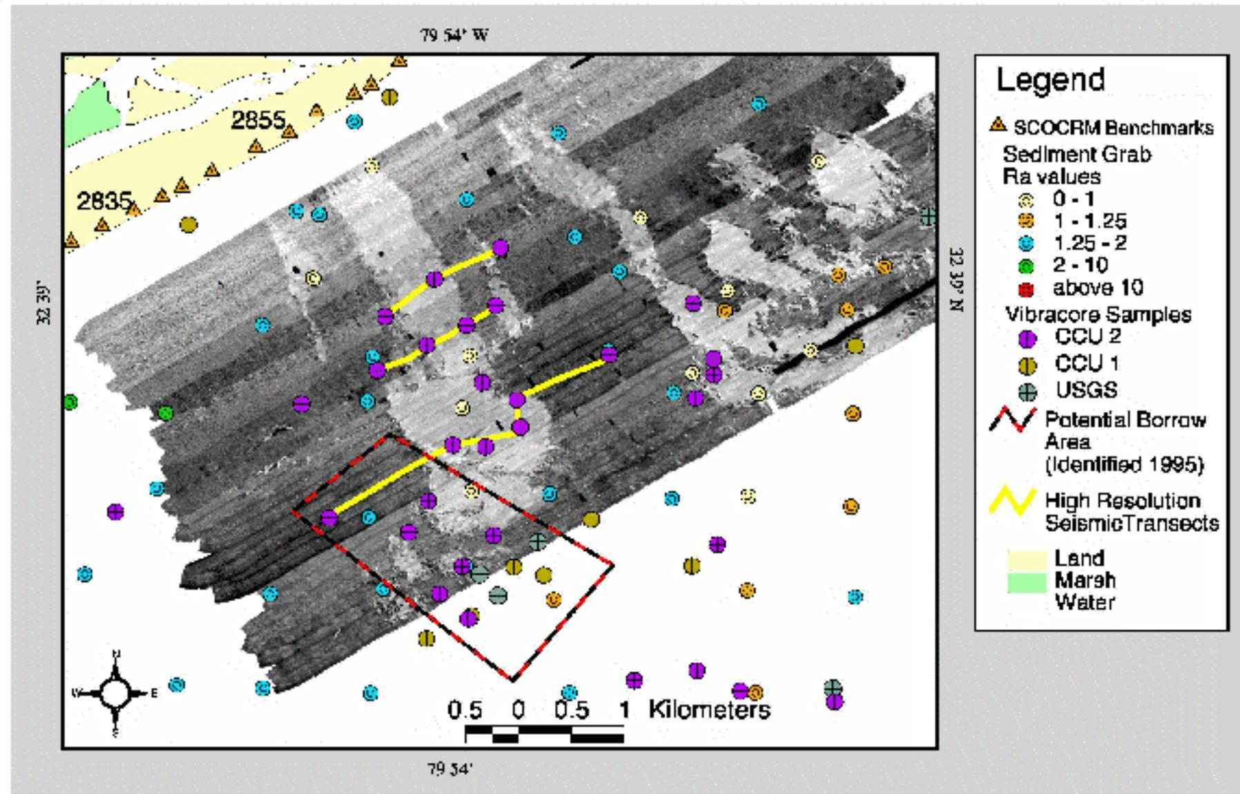
Figure 2. Sediment sample and vibracore locations superimposed on 1995 side scan sonar mosaic. Sample numbers and textural data are provided in Figures 7, 13 and 15 and Appendices 1, 2 and 3.
