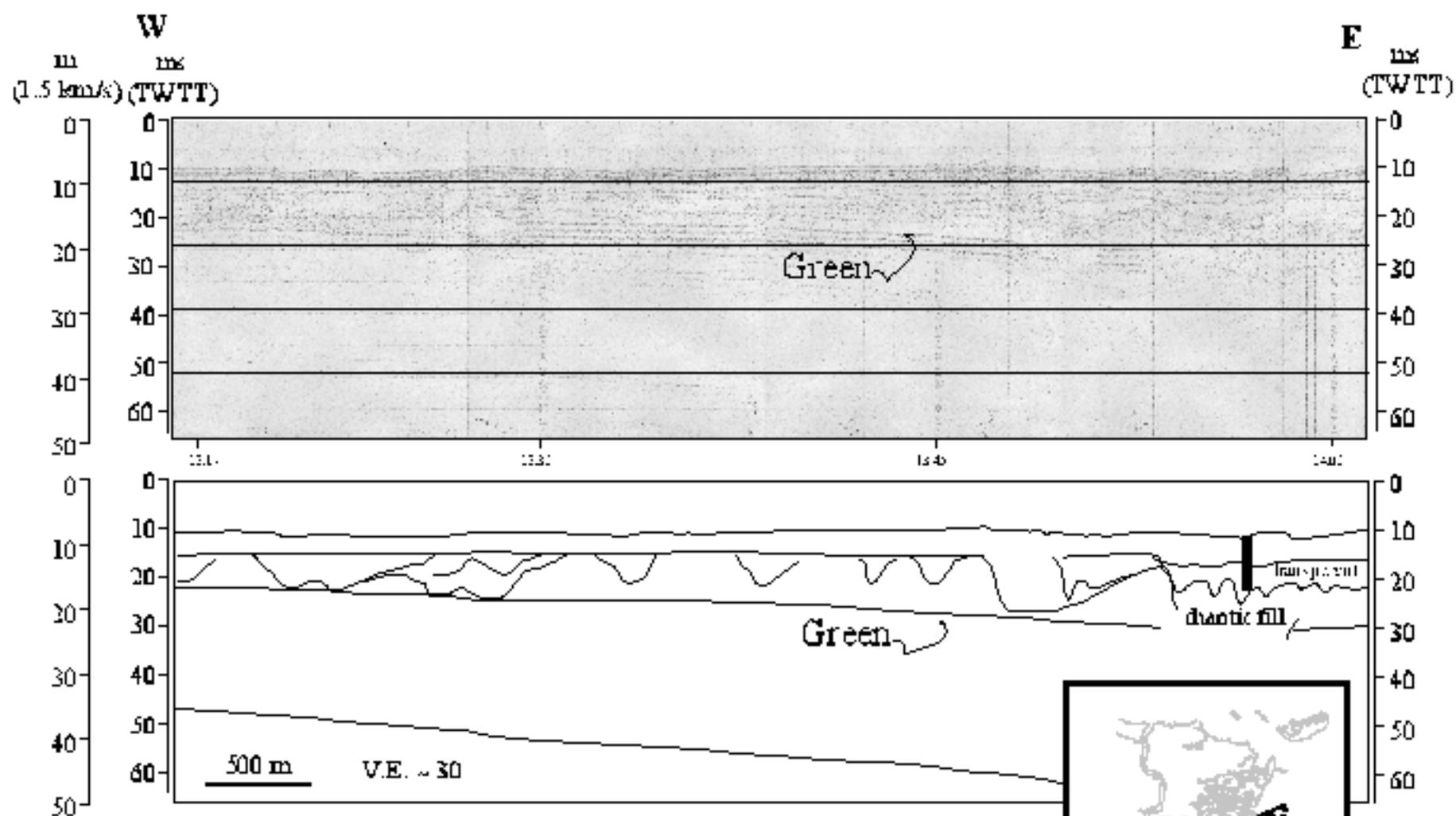
Figure 9. Interpreted seismic reflection profile from the inner shelf off Folly Beach, South Carolina. The profile illustrates the nature of the shallow subsurface stratigraphy.
