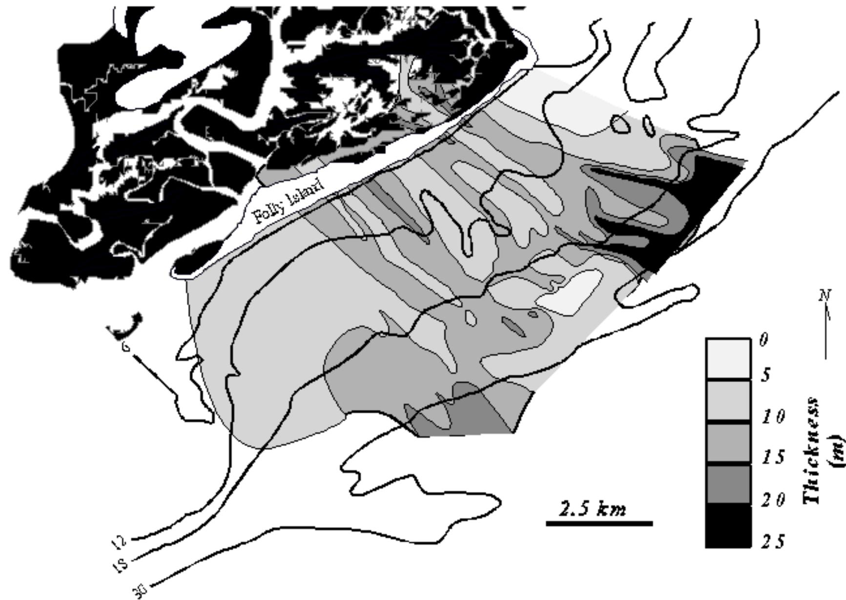
Figure 11. This isopach (thickness) map of Quaternary deposits indicates the presence of a Tertiary high spot beneath the shoreface. Thickness deposits to the northeast fill a Holocene paleovalley. Small incisions to the southeast of the Tertiary high are filled with paleochannel materials. Bathymetric contours in feet below mean sea level.
