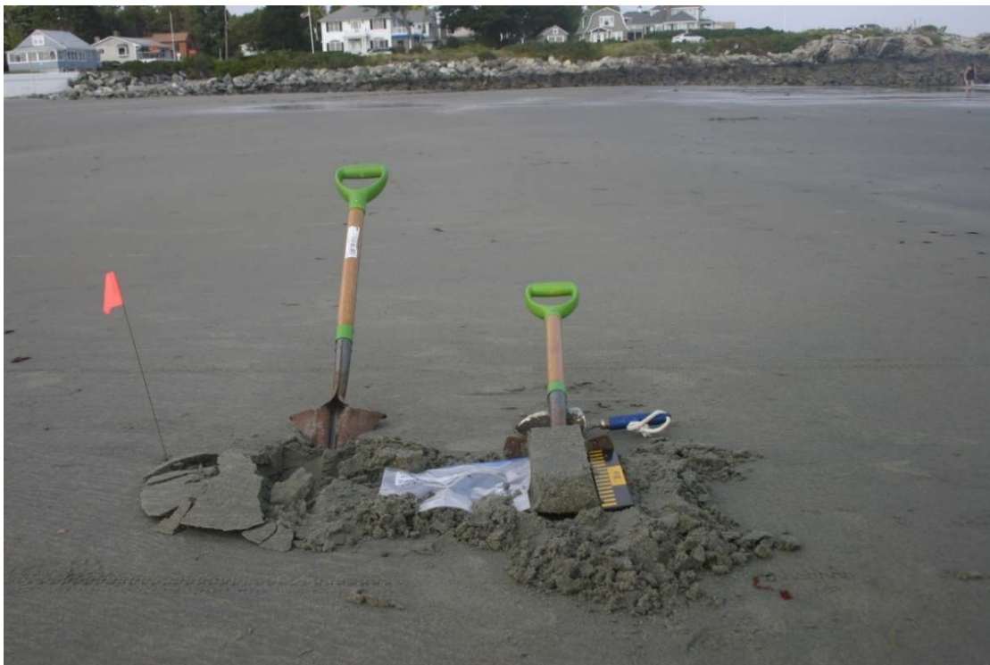
Figure 5-2. Collection of a beach sediment core at Wallis Sands station WS01 on September 5, 2017.
