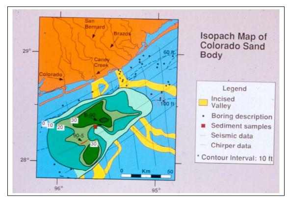
Figure 8. Isopach map (in feet) of the offshore Colorado River delta.
