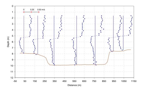
Figure 3.17 Representative Velocity Profiles for North-South Transect Line (05-Mar-2007 22:51-22:58 CST)
