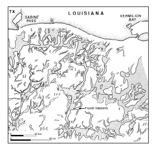
Figure 7. Map showing the distribution of late Wisconsin, incised fluvial systems offshore of the western Louisiana Chenier Plain. Location of the map is shown in figure 1 (from Suter et al., 1987).
