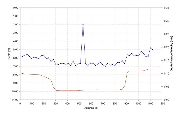
Figure B.2.26 Depth-Average Flow Velocity Change Across North-South Cross-Section (File no. 162819)
