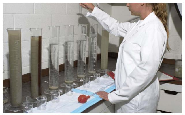
Figure A5 Mixing silt and clay as part of pipette analysis to determine silt and clay contents
