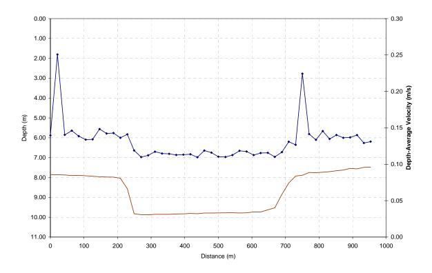
Figure B.2.33 Depth-Average Flow Velocity Change Across Diagonal Cross-Section (File no. 142104)
