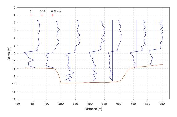
Figure B.2.17 Velocity Profiles for Diagonal Transect Line (File no. 142104)
