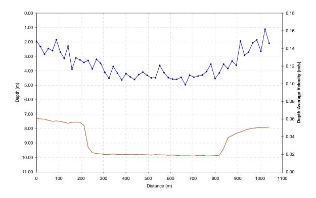
Figure B.2.25 Depth-Average Flow Velocity Change Across North-South Cross-Section (File no. 143243)
