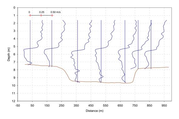
Figure B.2.21 Velocity Profiles for Diagonal Transect Line (File no. 184830)
