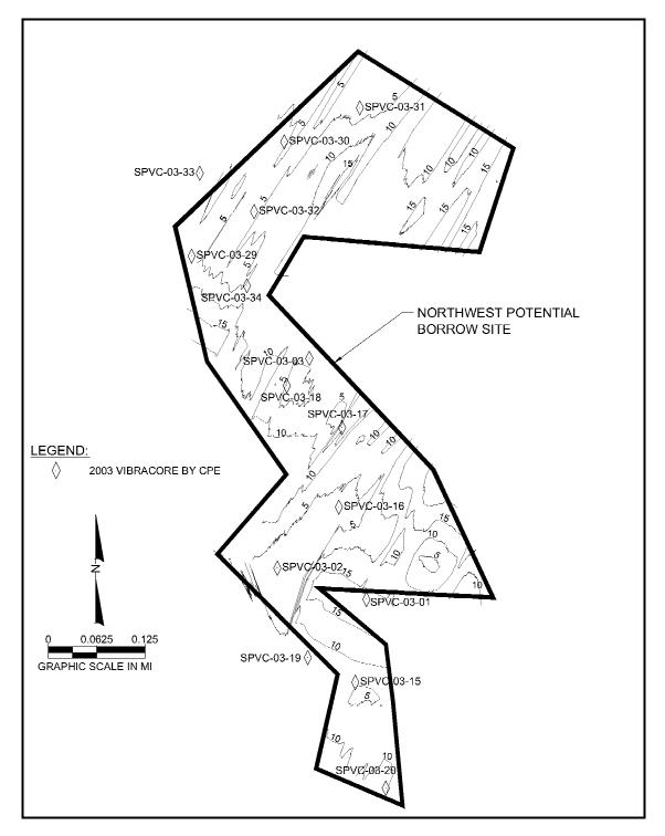
Figure 23. Map of the northwestern borrow site that shows the thickness of the overburden as determined by CPE (2002) from vibracores and seismic profiles. Contours are in feet.
