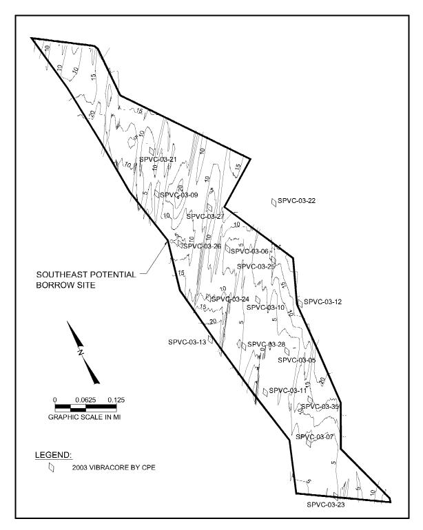
Figure 26. Map of the southeastern borrow site that shows the thickness of the overburden as determined by CPE (2002) from vibracores and seismic profiles. Contours are in feet.
