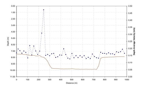
Figure 3.25 Depth-Average Flow Velocity Change Across Diagonal Cross-Section (05-Mar-2007 23:04-23:11 CST)
