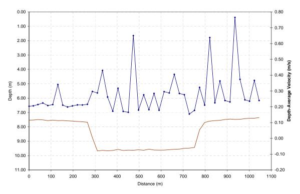
Figure B.2.32 Depth-Average Flow Velocity Change Across East-West Cross-Section (File no. 3629)
