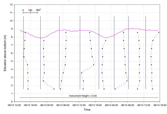
Figure 3.16 Current Direction Profiles for Holly Beach Site 7, June 2006 ("direction to" is plotted)
