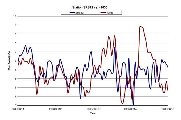
Figure 3.40 Wind Data Recorded at the Two Stations During the Period of Model Calibration
