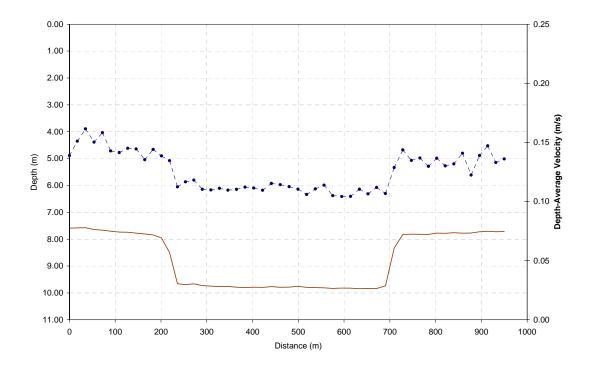
Figure 3.24 Depth-Average Flow Velocity Change Across East-West Cross-Section (05-Mar-2007 20:33-20:40 CST)
