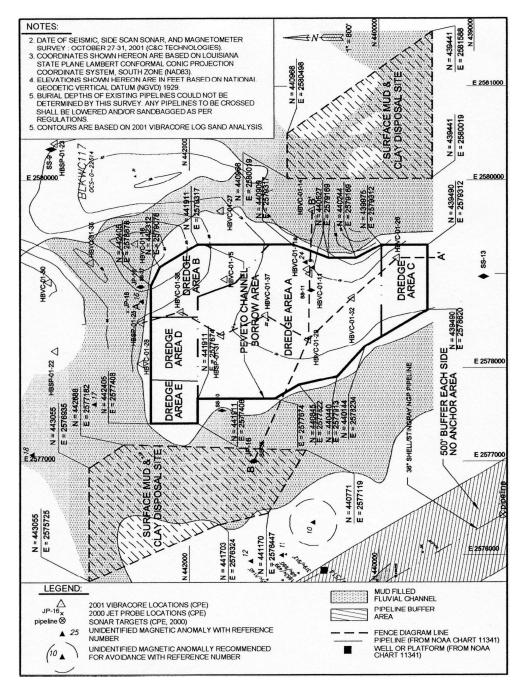
Figure 14. Close-up map of the sand body L (shown in figure 13) with the designated targets within the location. Lines of cross section (A to A'; B to B') are shown for figures 15 and 16.
