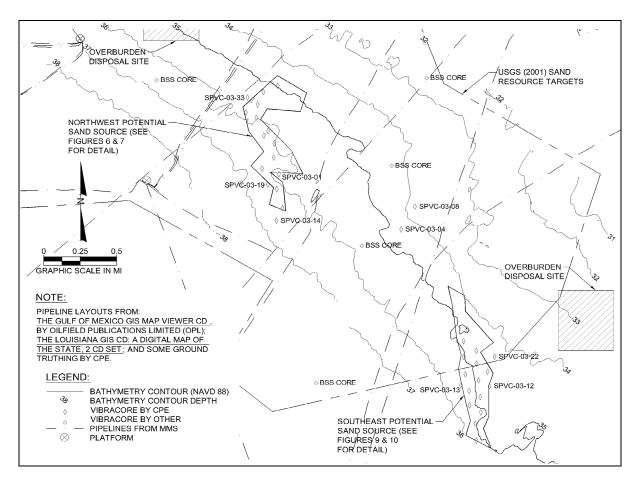
Figure 20. Base map of the Sandy Point area showing the bathymetry determined by CPE (2002) as well as the distribution of cores obtained during their investigation. (SPVC-03; BSS cores from Kindinger et al., 2002).
