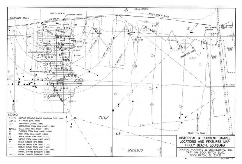
Figure 8. Base map from CPE (2002) showing the distribution of vibracores, jet probes, and high- resolution seismic profiles in the Pevoto Beach Channel deposit.
