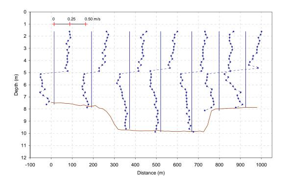
Figure 3.21 Representative Velocity Profiles for Diagonal Transect Line (05-Mar-2007 23:04-23:11 CST)
