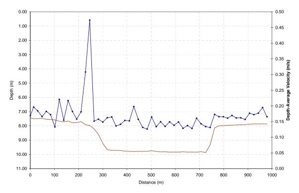
Figure B.2.34 Depth-Average Flow Velocity Change Across Diagonal Cross-Section (File no. 164148)
