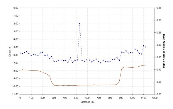
Figure 3.23 Depth-Average Flow Velocity Change Across North-South Cross-Section (05-Mar-2007 22:51-22:58 CST)
