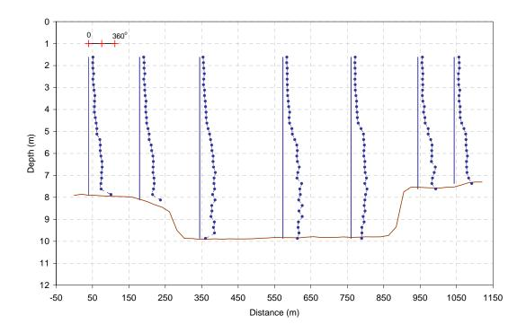
Figure 3.18 Representative Direction Profiles for North-South Transect Line (05-Mar-2007 22:51-22:58 CST) ("direction to" is plotted)
