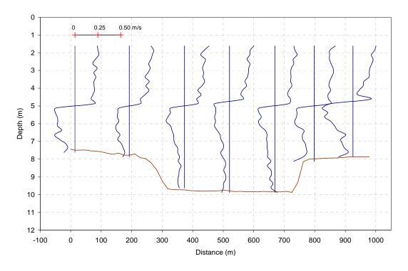
Figure B.2.19 Velocity Profiles for Diagonal Transect Line (File no. 164148)
