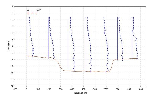
Figure 3.22 Representative Direction Profiles for Diagonal Transect Line (05-Mar-2007 23:04-23:11 CST) ("direction to" is plotted)
