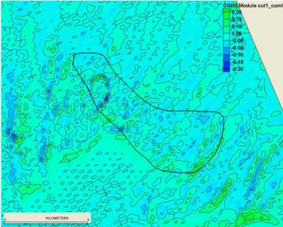
Figure 4-71. Topographic change over shoal A8 after two years of simulation with a single borrow excavation located on the crest (Case 8).
