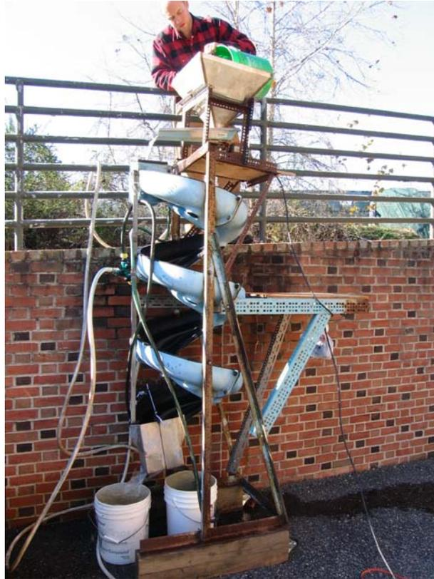
Figure 1. Three-turn Humphrey Spiral: Heavy mineral concentrate is collected in the bucket to the right.
