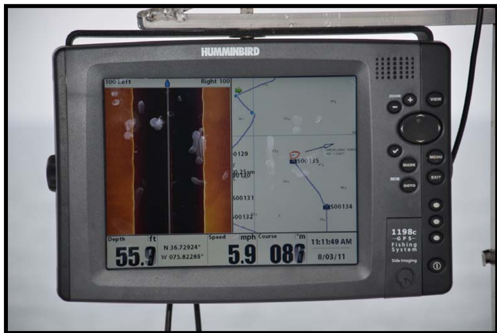
Figure 2 - Side scan sonar unit aboard the Matador
