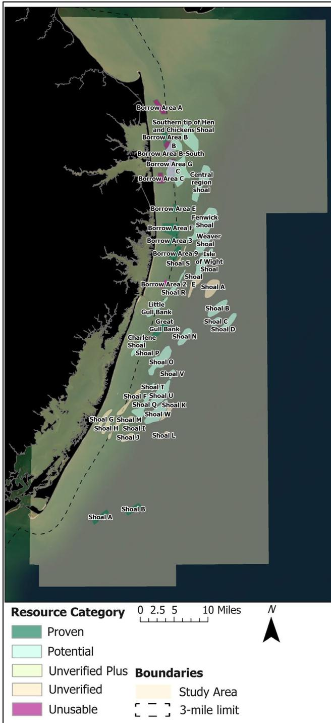
Figure A-1. Overview of known borrow areas and shoals from the BOEM Data Center. Borrow areas are categorized based on how well they have been characterized by core data, geophysical surveys, and past usage.
