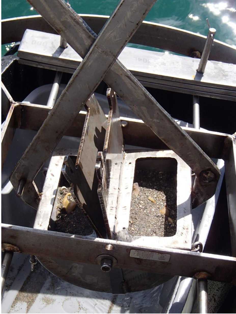
Figure 11-4. Young grab with doors of the van Veen grab open, showing sediment capture.
