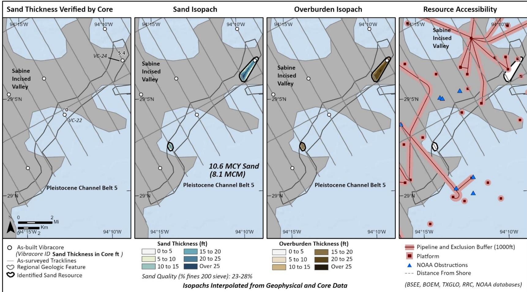
**Figure 26. Panel figure of sand sampled in cores, identified sand resources, overburden, and accessibility of Pleistocene Fluvial North Terrace.**
