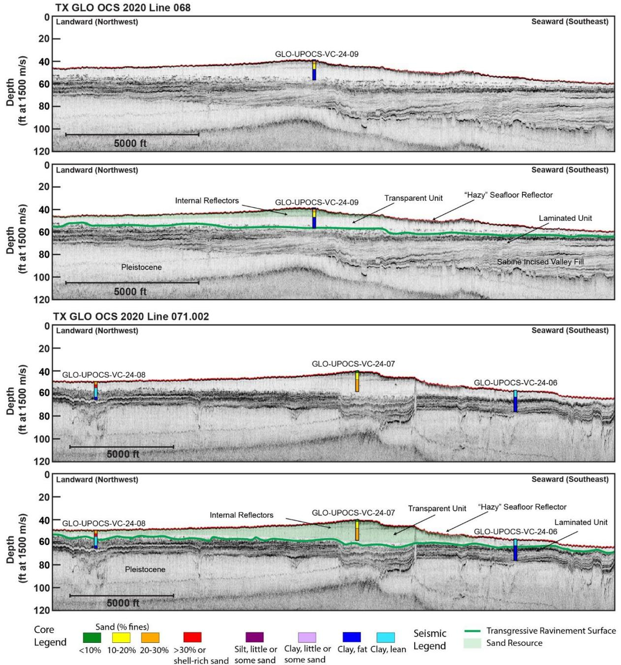
Figure 13. Example sub-bottom data across the Shepard Bank flanking shoals, demonstrating the thickness of Q1 surficial sand deposits likely extending beyond the investigation area. See Figure 7 for location. Inset Figure 33 shown in Localized Feature section.
