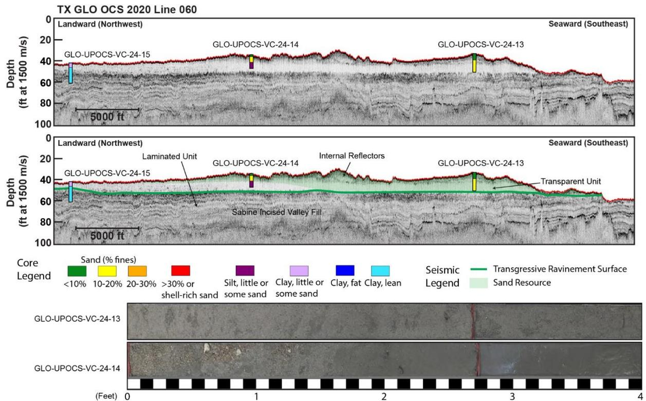
**Figure 12. Example sub-bottom data across Shepard Bank flank displaying the sediment composition variability of similar transparent seismic facies. See Figure 7 for location.**
