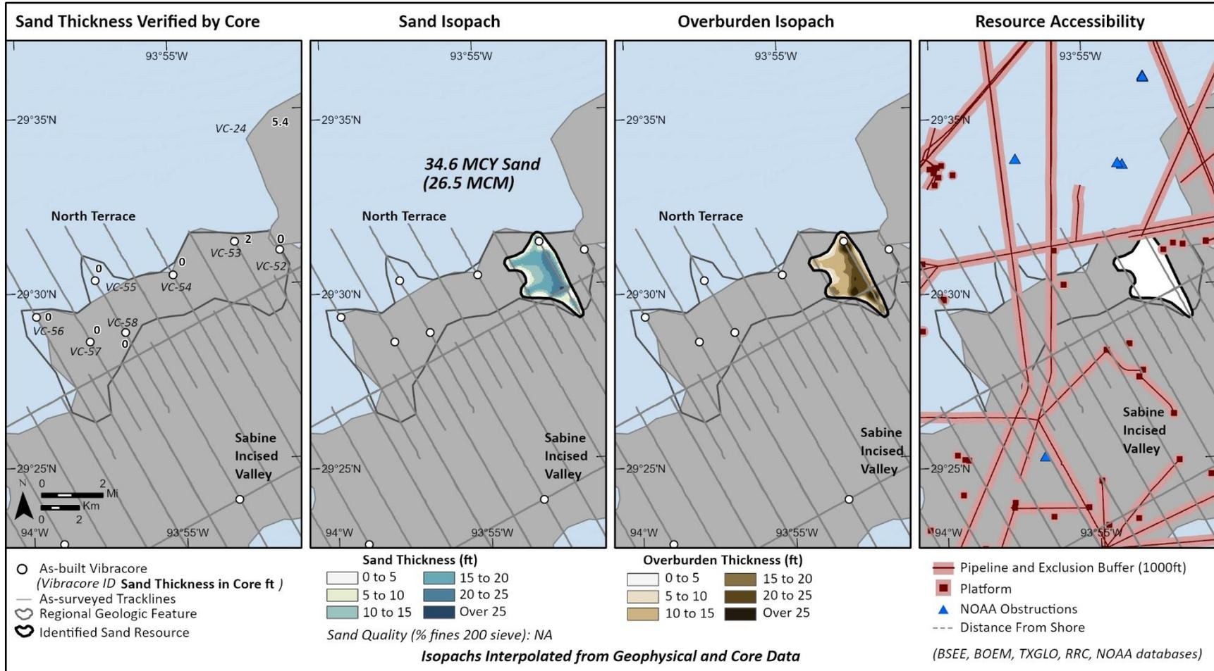
**Figure 27. Panel figure of sand sampled in cores, identified sand resources, overburden, and accessibility of Pleistocene Fluvial South Terrace.**
