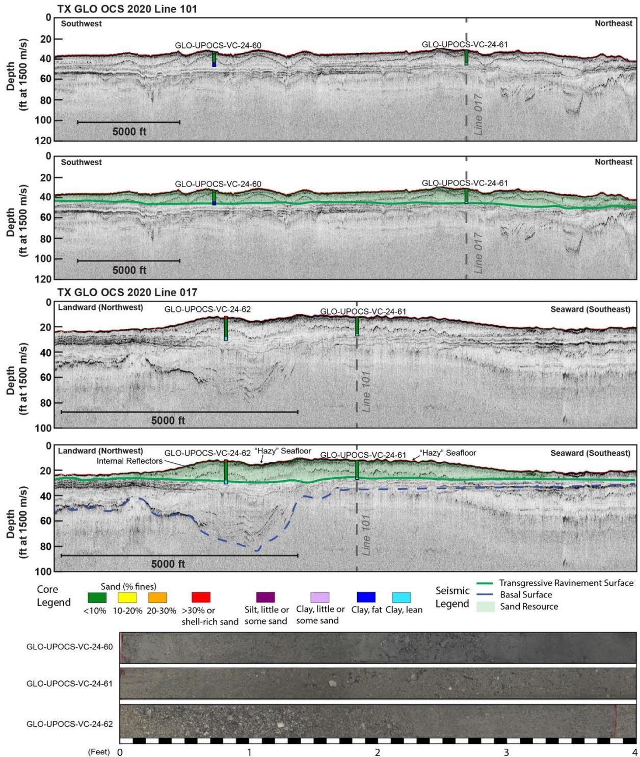
Heald Bank is an overall lunate-shaped shoal, with the thickest portion located at the central crest and tapering on its flanks. Transects of vibracores obtained through the central bank crest and the flanks detail its sand resource potential and variable composition. The central portion of Heald Bank contains over 15
