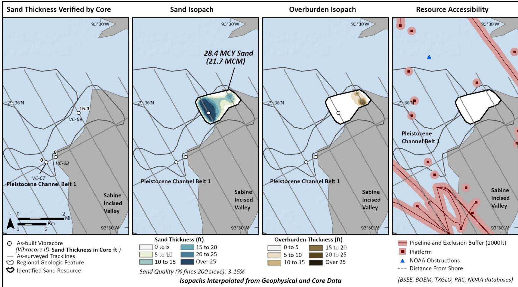
**Figure 24. Panel figure of sand sampled in cores, identified sand resources, overburden, and accessibility of Pleistocene Channel Belt 2.**
