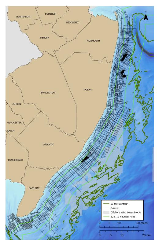
Ninety-foot water depth contour, which reaches a maximum of 18nm offshore at the farthest point. This water depth corresponds to the typical operational limit of U.S.-flagged sand dredges and has been largely unexplored for sand resource potential. Also shown are NJGWS and BOEM offshore seismic track lines and federal wind lease blocks.
