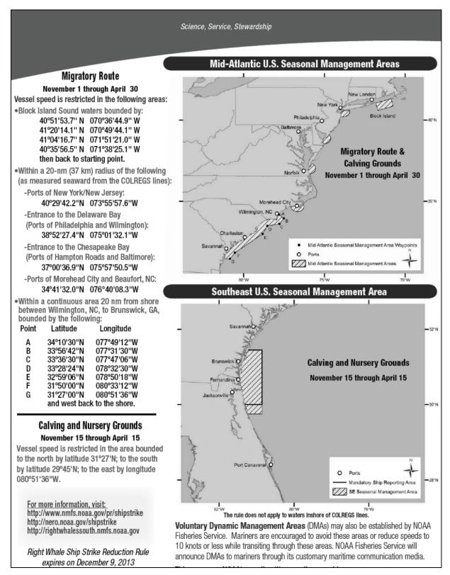
Figure 2-1. Summary of Speed Restrictions and Locations for Vessel Operators to Comply with the Right Whale Strike Reduction Rule (50 CFR § 224.105) (USDOC, NOAA, 2011).
