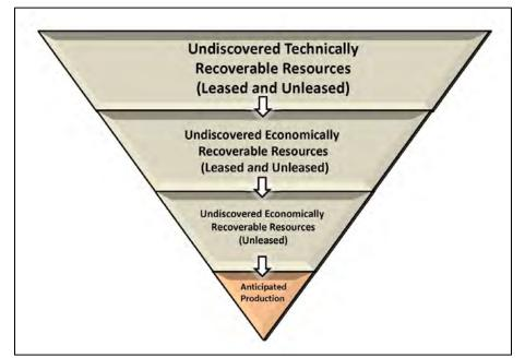
Figure 5-4: Conceptual Workflow Showing Transition from UTRR to Anticipated Production
