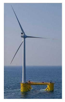
Figure 3 - WindFloat Prototype
