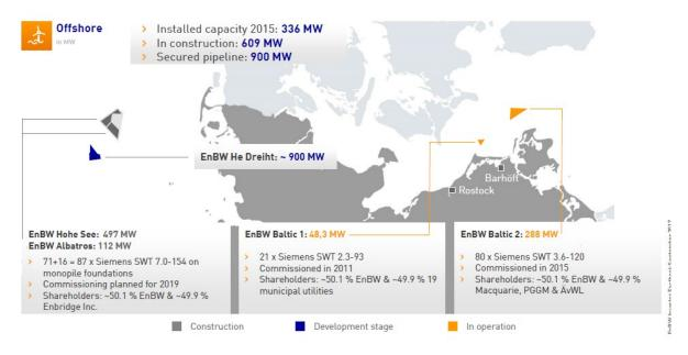
Figure 7 EnBW's Offshore Wind Assets
