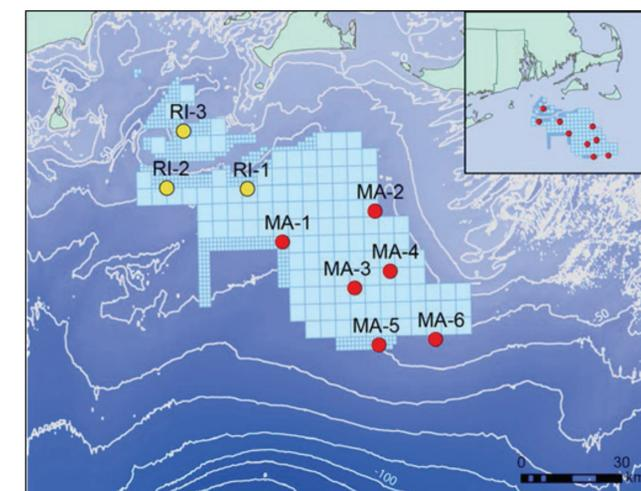
Recording sites (red and yellow dots) in the MA and RI wind energy areas, from November 2011 to March 2015. Ambient sound levels across all sites varied between 96 dB and 103 dB re 1  $\mu$ Pa in the hearing range of baleen whales during 50% of the recording time. These measurements were part of a cooperatively funded study by BOEM and MassCEC. ([www.boem.gov/RI-MA-Whales-Turtles](http://www.boem.gov/RI-MA-Whales-Turtles))
