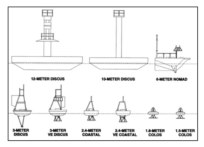
**Figure 3-7. Buoy Schematic** Source: National Data Buoy Center, 2008.
