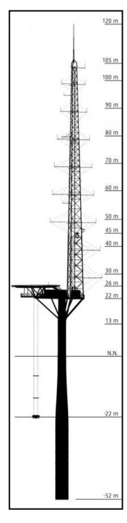
Figure 4-16. Elevation Diagram of FINO 3 Meteorological Tower Schematic diagram available at: http://www.fino3.de/en/fino3/design-of-the-fino3.
