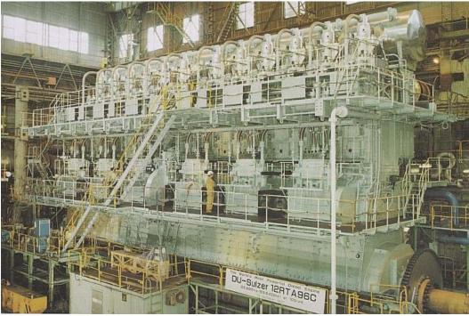
Figure C-2. Photograph of the Wärtsilä-Sulzer RTA96-C two-stroke marine diesel engine for the Emma Maersk (Denmark).
