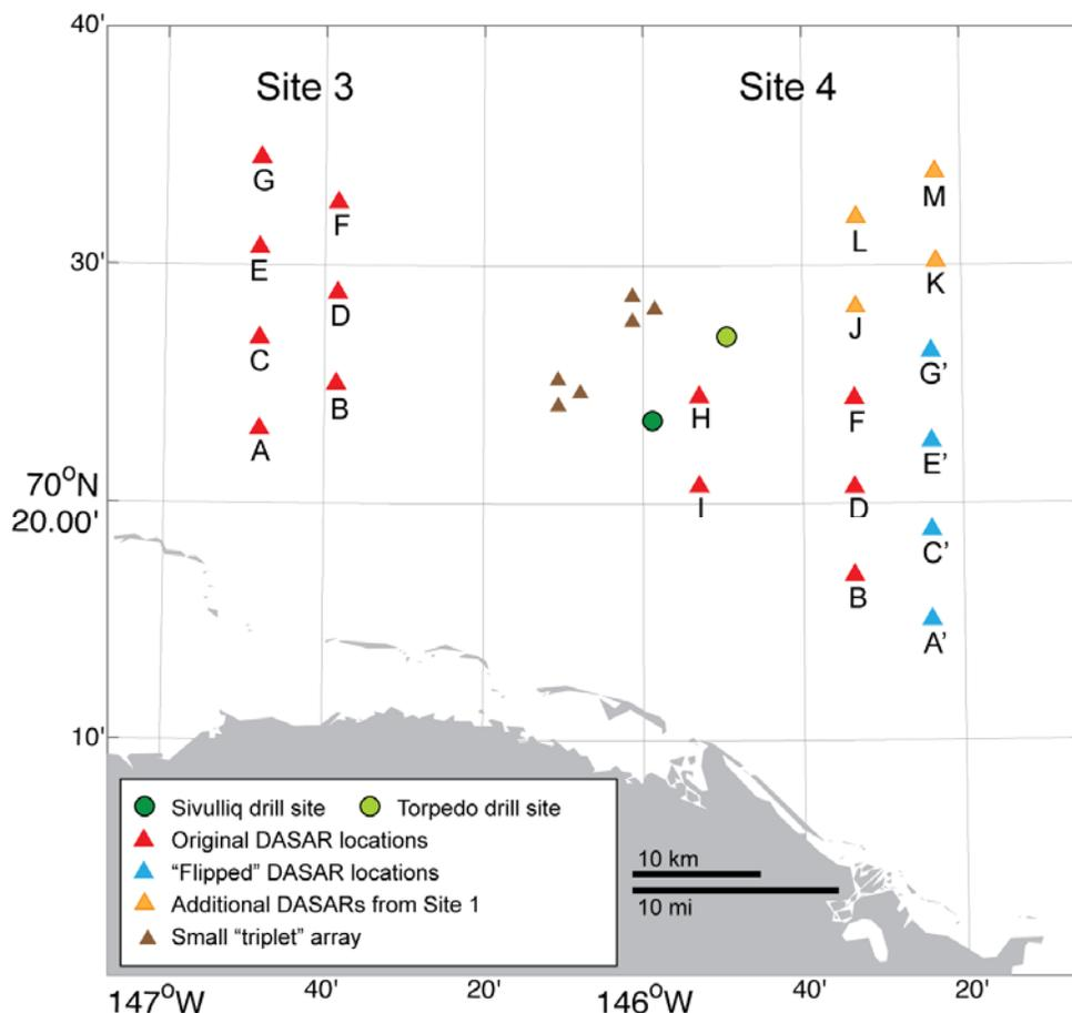
Figure 5. DASAR deployments at sites 3 and 4. DASARs are shown with triangles and the two drill sites, Sivulliq and Torpedo, are shown with green dots. The drill sites will be used consecutively. The triplets of DASARs (small brown triangles) will be retrieved when and if the drillship is moved and redeployed in the new location in the same relative positions. All other DASARs will remain in place over the entire season.
