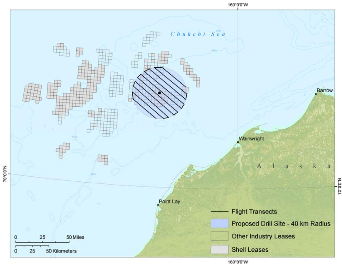
Figure 8. Aerial photographic survey design for the Chukchi Sea drill sites. This design maximizes the area covered in a single flight and assumes 7.2 km between transect lines.
