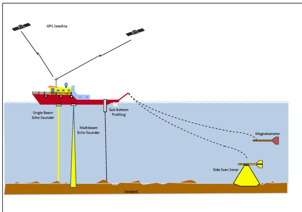
Figure 2.2-1 Schematic of Ice Gouge Survey Acquisition
