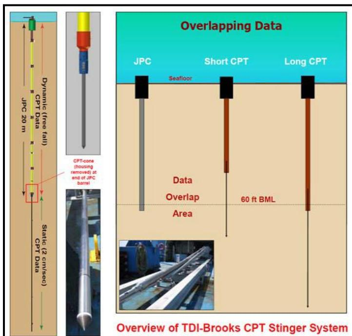
**Figure 2.3-2 Schematic of Geotechnical Survey Acquisition with Piston Core / CPT System**
