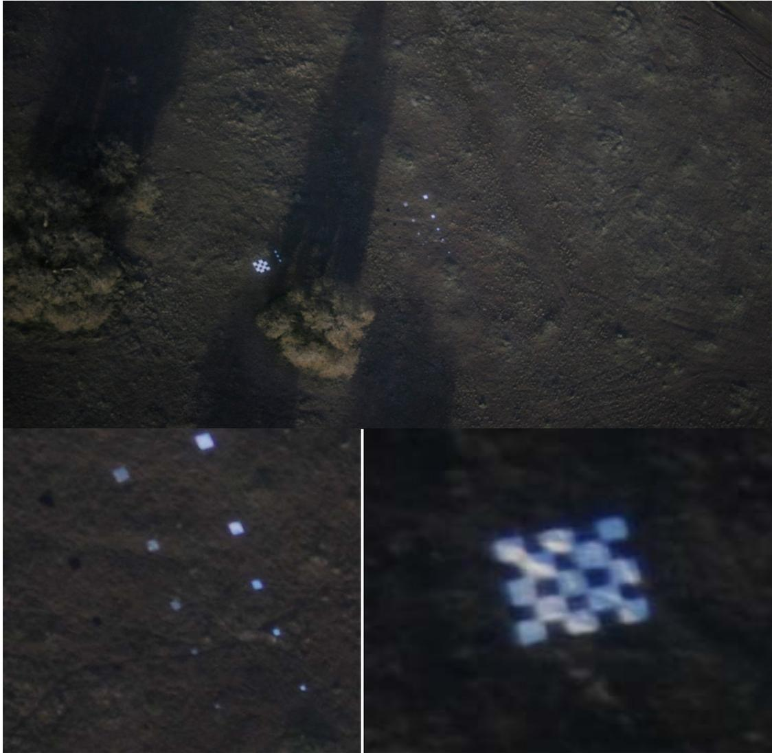
Figure 6. Photograph taken from an UAS during resolution tests at Camp Roberts, California, during December 2009. The upper photographs were taken with a 12 megapixel camera with resolution on the ground of 2.9 cm. The colored patches in the lower left photograph vary in size from 15 cm squares to 50 cm squares and are a magnified view of the upper photograph. The lower right photograph is a magnified view of a 2 m square checkerboard with each checkerboard square 40 cm by 40 cm.
