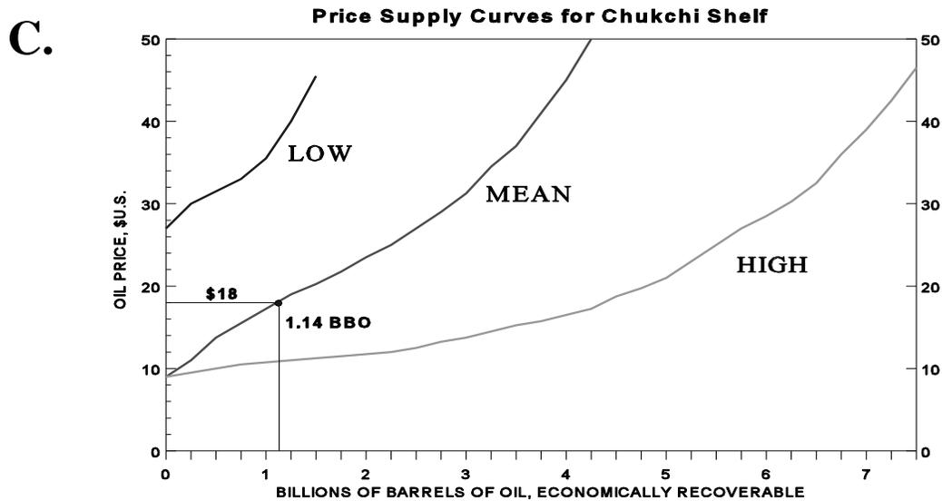
**Figure 4:** Chukchi shelf assessment province. (A) Cumulative frequency distributions for risked, undiscovered conventionally recoverable resources; (B) Table comparing results for conventionally and economically recoverable oil and gas; (C) Price-supply curves for oil at low (F95), mean, and high (F05) resource cases. BOE, total oil and gas in billions of energy-equivalent barrels; MPhc, marginal probability of hydrocarbons for basin; BBO, billions of barrels; TCFG, trillions of cubic feet.
