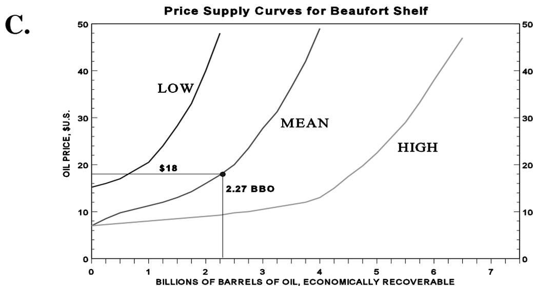
**Figure 3:** Beaufort shelf assessment province. (A) Cumulative frequency distributions for risked, undiscovered conventionally recoverable resources; (B) Table comparing results for conventionally and economically recoverable oil and gas; (C) Price-supply curves for oil at low (F95), mean, and high (F05) resource cases. BOE, total oil and gas in billions of energy-equivalent barrels; MPhc, marginal probability for hydrocarbons for basin; BBO, billions of barrels; TCFG, trillions of cubic feet.
