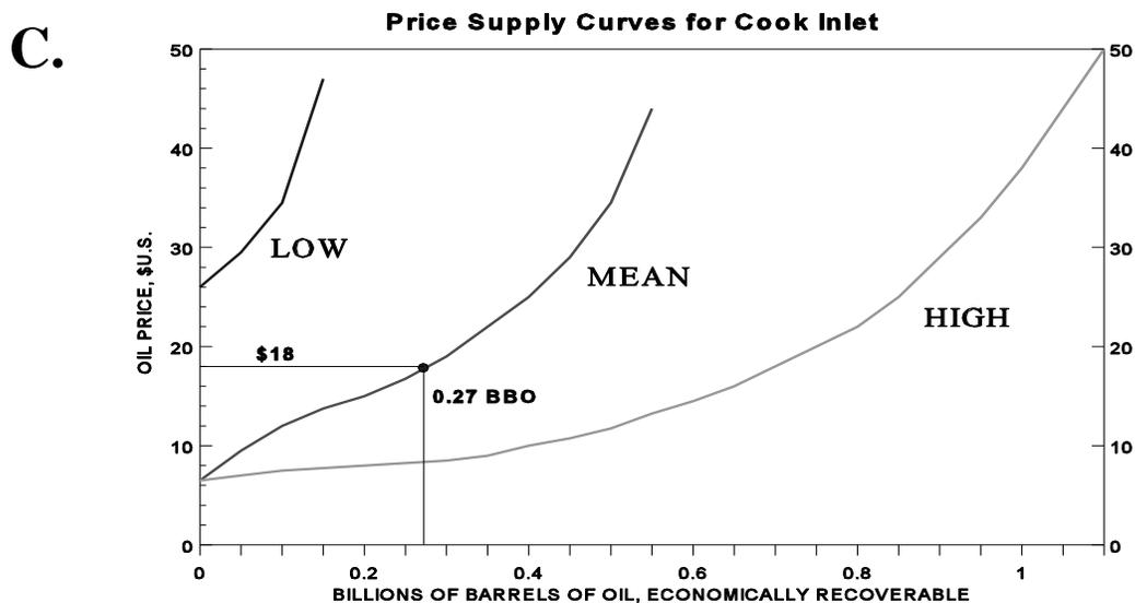
**Figure 5:** Cook Inlet assessment province. (A) Cumulative frequency distributions for risked, undiscovered conventionally recoverable resources; (B) Table comparing results for conventionally and economically recoverable oil and gas; (C) Price-supply curves for oil at low (F95), mean, and high (F05) resource cases. BOE, total oil and gas in billions of energy-equivalent barrels; MPhc, marginal probability for hydrocarbons for basin; BBO, billions of barrels; TCFG, trillions of cubic feet.
