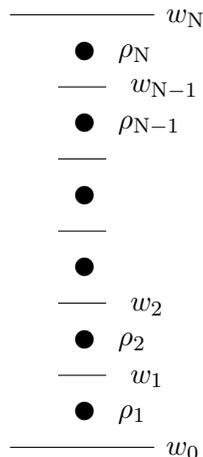
Figure 2: Placement of variables on staggered vertical grid
