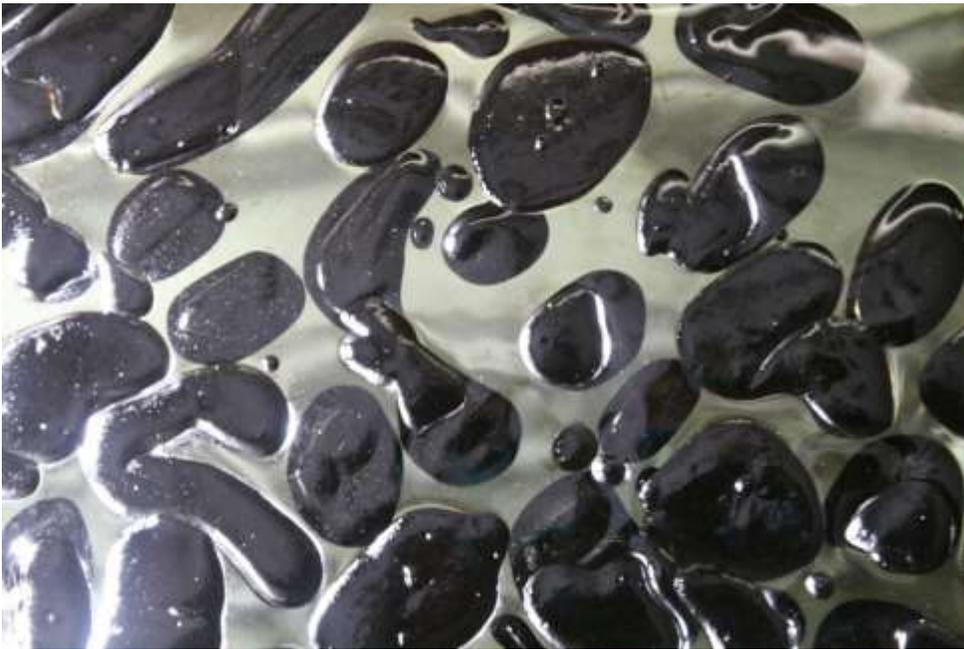
Sample 9 –72 hours weathering. The blackish lumps observed in the meso-scale flume are typical for asphaltenic crude oils.
