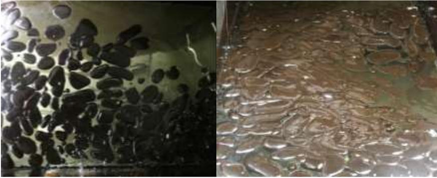
Sample 8 –48 hours (emulsion color changes due to direct exposure to solar simulator, right)
