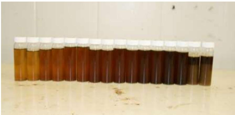
Figure 4.4. The oil-samples Sample 1 (0.5 hour) – Sample 8 (48 hours) from left to right with observed changes in the color appearance over time
