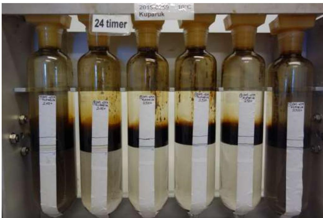
Figure 3.11. The rotating cylinders of water-in-oil emulsion of Kuparuk crude oil after 24 hours of rotation at 10 °C, given as example for the 200 and 250°C+ residue
