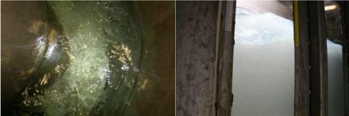
Sample 0 (Start)—Application of ADO – Natural dispersion started immediately when wave action was turned on.
