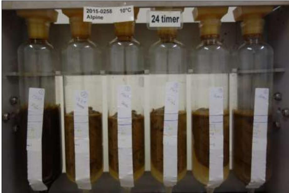
Figure 3.9. The rotating cylinders of water-in-oil emulsion of Alpine crude oil after 24 hours of rotation at 10 °C
