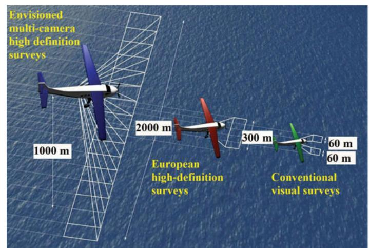
Comparison of aerial high-definition survey flight heights. Image courtesy of Normandeau Associates and Boulder Imaging.
