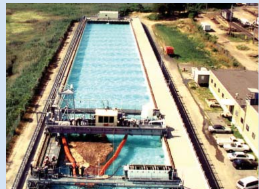
Above: Oil containment boom being tested with oil in waves Left: Breaking waves generated at OHMSETT.
