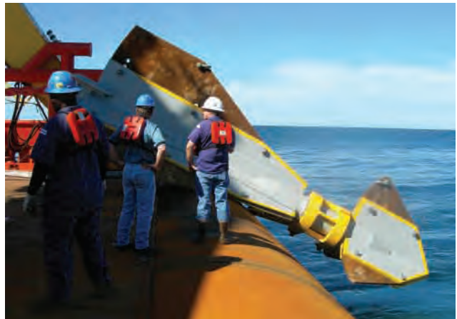
Anchor used for mooring of mobile offshore drilling unit (MODU). Since Hurricanes Katrina and Rita, the type of anchor used will get special consideration since it can be critical to the amount of damage a platform incurs when a hurricane strikes.
