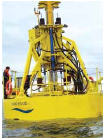
The Wavebob is an axi-symmetric, self-reacting point absorber, operating mainly in the heave mode. Developed by an Irish company, Wavebob, Ltd., it is specifically designed to recover useful power from ocean wave energy and to be deployed in large arrays offshore. In 2008 Wavebob, Ltd. received the Green Innovation Award in Dublin. Photo courtesy of wavebob.com.
