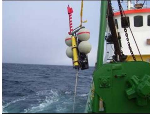
Figure 3. Hydrophone recording system being deployed at sea. The hydrophone system is an autonomous recorder with very high recording resolution. Acoustic data is stored internally on a hard-drive.
