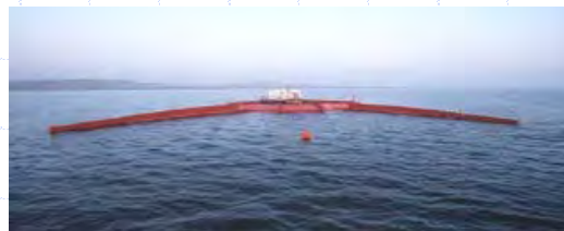
Overtopping -Wave Dragon
