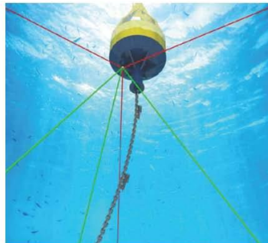
A standard current profiler cannot measure the complete profile from the bottom to the surface. Instead, it loses data close to the instrument and close to the far boundary. The Aquadopp Z-Cell extends the profiling range by introducing a «Cell Zero». The data is generated by an extra set of horizontal transducers. The transducers operate at a different frequency (2 MHz) and provide the 2D current velocity at the level of the instrument. This is to the benefit of anyone who is interested in the detailed current velocity in the boundary layer.
